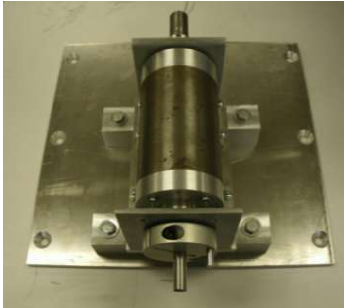
Figure 4.14. PMSG built based on the RMxprt design
