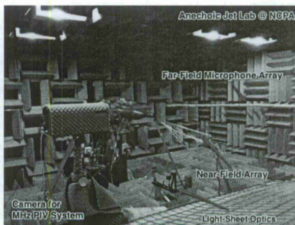
FIGURE 2. The NCPA Anechoic Jet Laboratory setup for the simultaneous near-field/far-field/MHz-PIV measurements.
