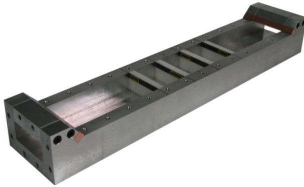
Figure 2.4: WR-137 test fixture (cover plate removed) with SRR elements arranged for the SWA array.
