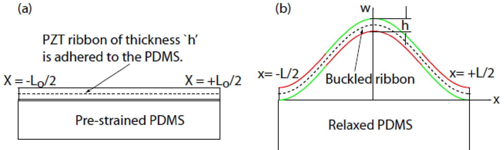
$$U^{bend} = \int_{-\frac{L_0}{2}}^{+\frac{L_0}{2}} \frac{1}{2} \frac{Eh^3}{12} \left( \frac{d^2w}{dX^2} \right)^2 dX = \frac{Eh^3 \pi^4 A^2}{12 L_0^3},$$
