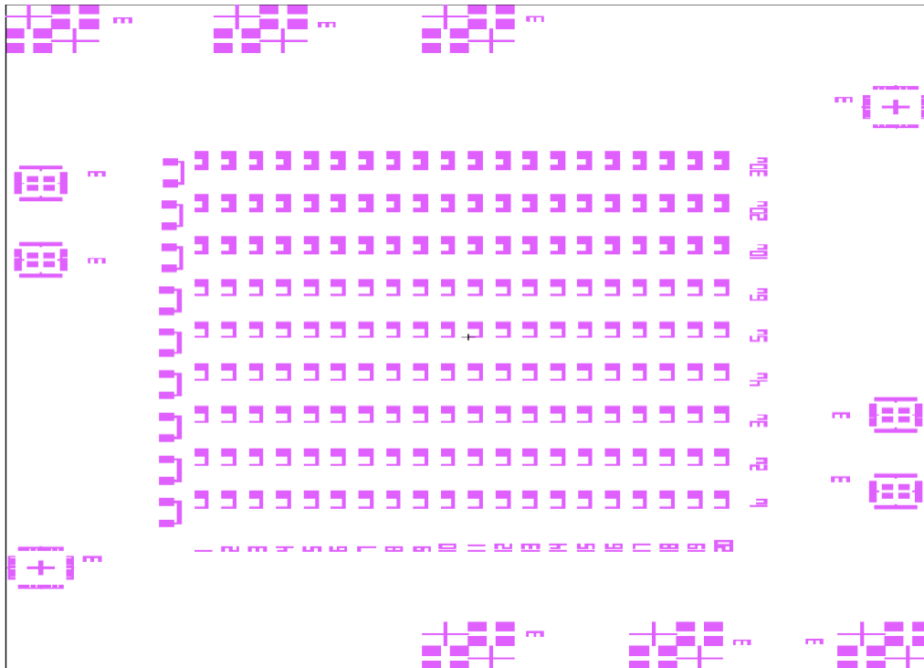
Fig. 36. Metal 2, Top Electrode (Mask 3).
