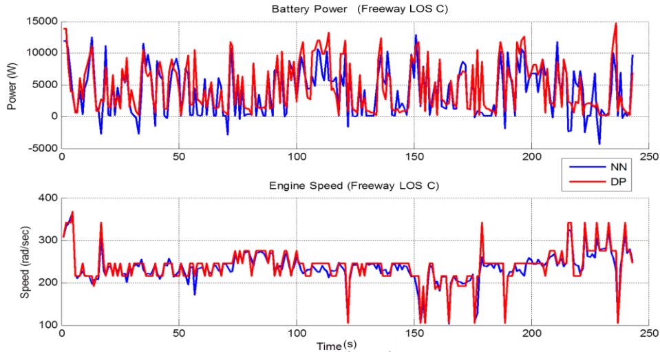
Figure 12. Comparison of optimal engine speed and battery power generated by the neural networks and DP for Freeway LOS C.
