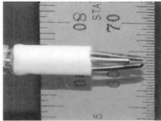
Figure 11: New Tungsten electrode design for high-speed applications.
