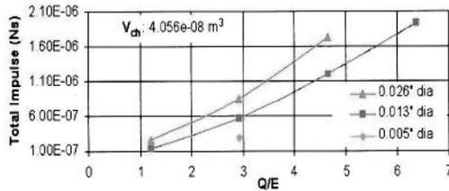
Figure 2: Effect of energy deposition on impulse.
