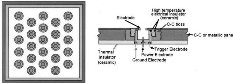
Figure 7: Integrated plasma device based on array of SparkJets.
