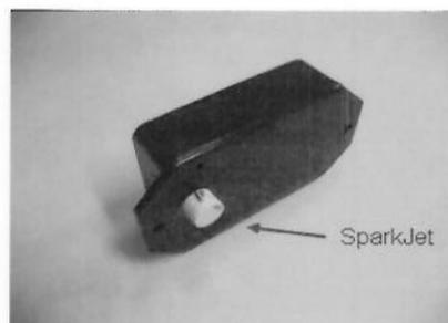
Figure 4: Individual SparkJet unit (with electronics, power supply).
