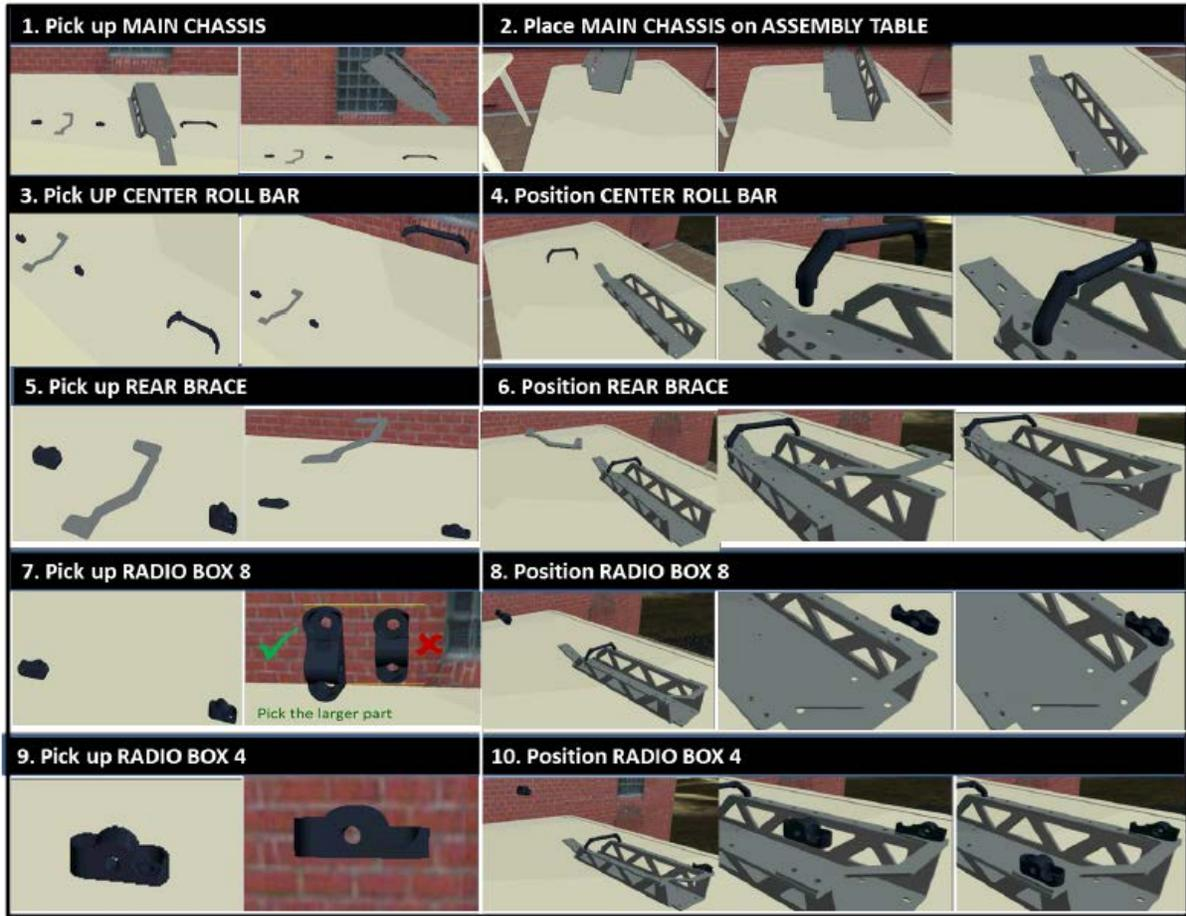
Figure UMD-18: Generated chassis-assembly instructions
