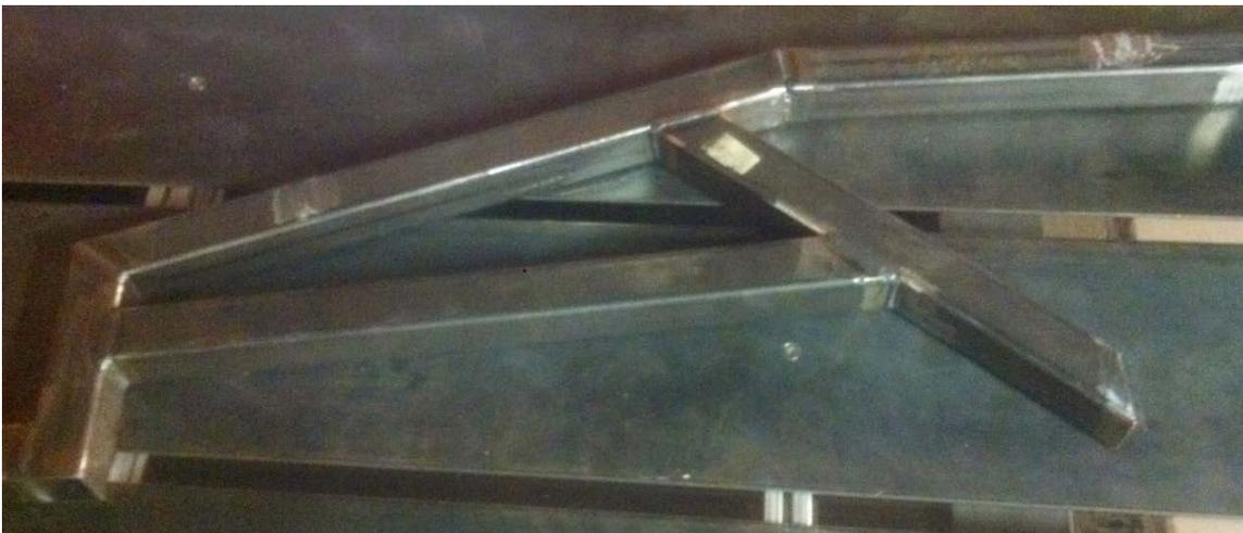
**Figure CMU-14: Hood-support subassembly**
