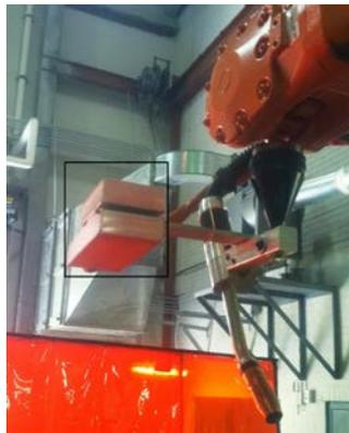
Figure CMU-8: Projector and sensor mounted on robot welding arm
