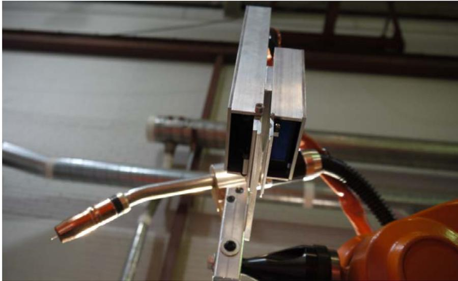
**Figure CMU-9: Robot Tooling –Projector (larger box) and displacement sensor (small box) lasers, mounted at an angle to the welding torch and off to the side**
