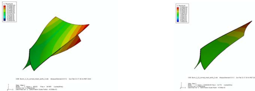
Mode 1. Frequency: 34.98 Hz
