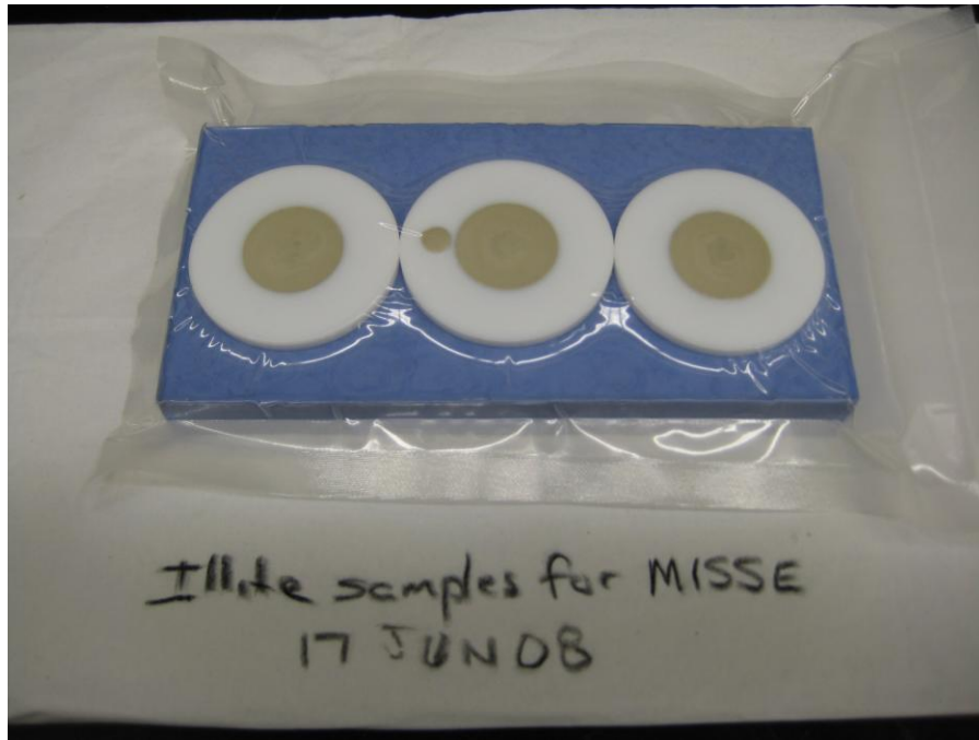
Illite samples prepared for MISSE-7 mission, vacuum bagged during cure, June 2008
