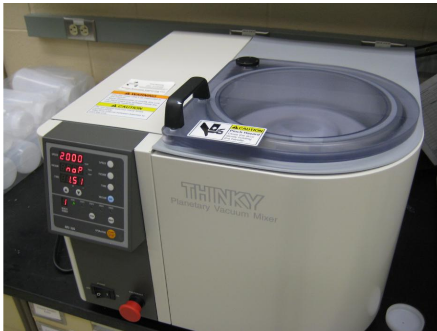
Figure 8. Thinky ARE-250 centrifugal mixer
