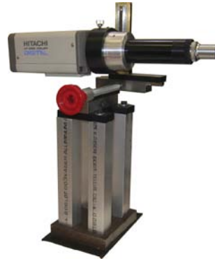
Figure D3 Custom-built long-working distant video microscope.
