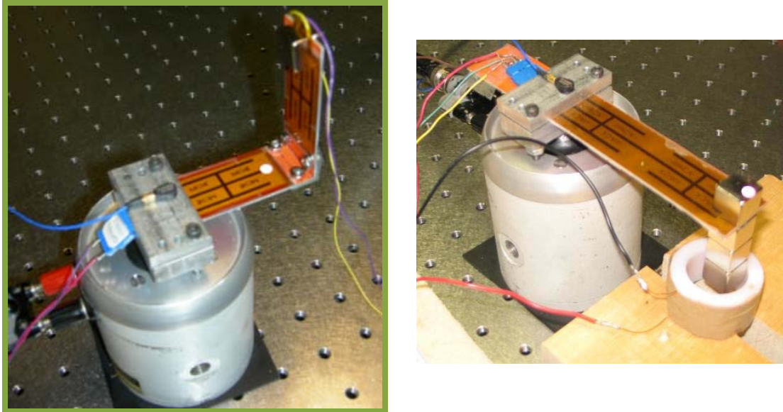
Figure G-3 On the right is the L-shaped configuration used to introduce nonlinear behavior and on the left is the combined piezoelectric and electromagnetic harvester.
