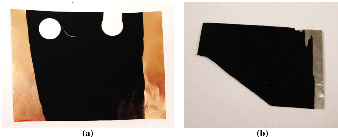
Figure D71. (a) Si anode sample (b) \text{LiCoO}_2 cathode sample.
