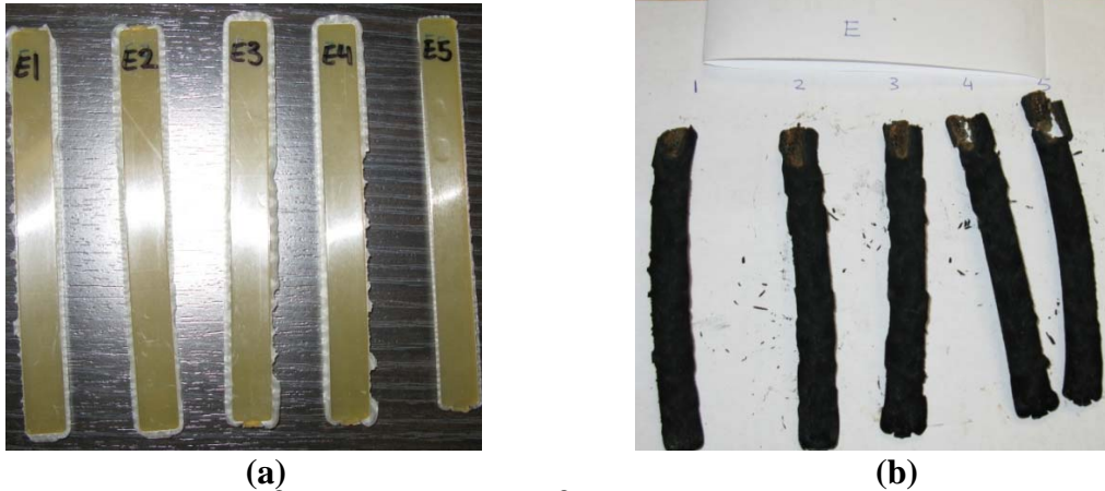
Figure 3.51 Desmopan ® + 10 wt% Cloisite ® 30B (a) before and (b) after vertical UL 94 test.
