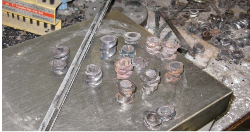
Figure 3.12 Screw sections of twin screw extruder.
