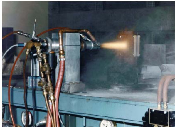
Figure 3.3 Texas State University-San Marcos simulated solid rocket motor.
