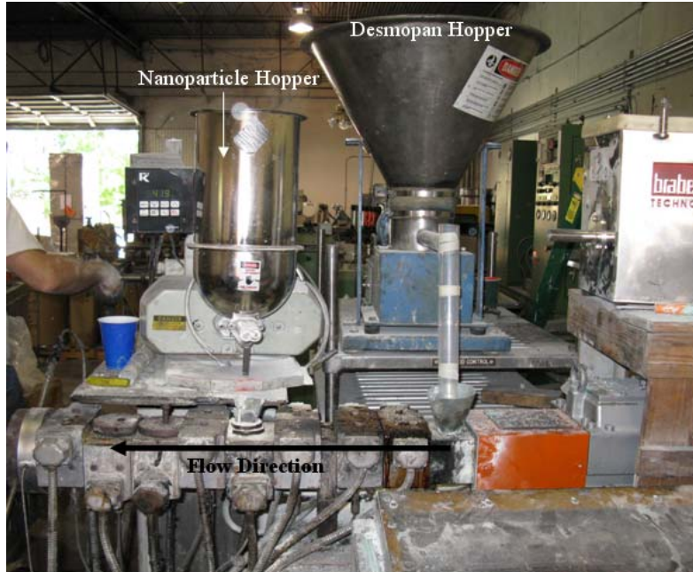
Figure 3.11 21 st Century Polymer twin screw extruder setup.
