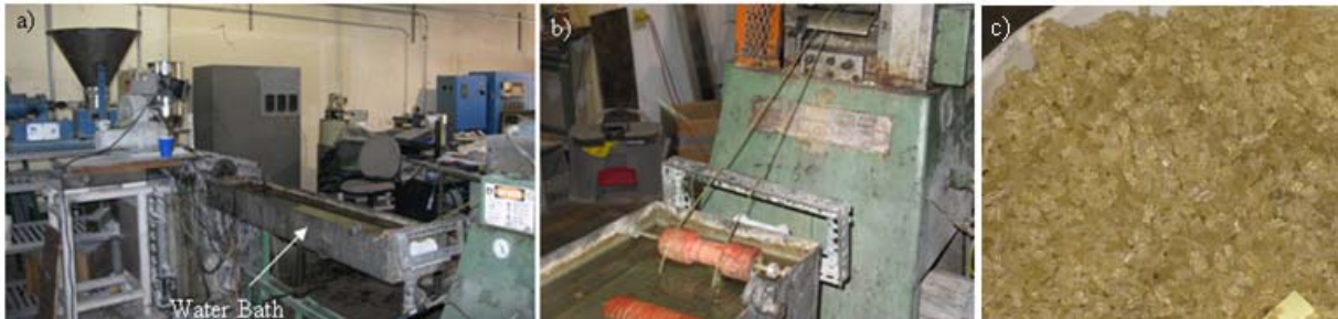
Figure 3.13 (a) - (c) (a) Water bath, (b) Machine used to cut polymer spaghetti into pellets, and (c) PNC pellets.
