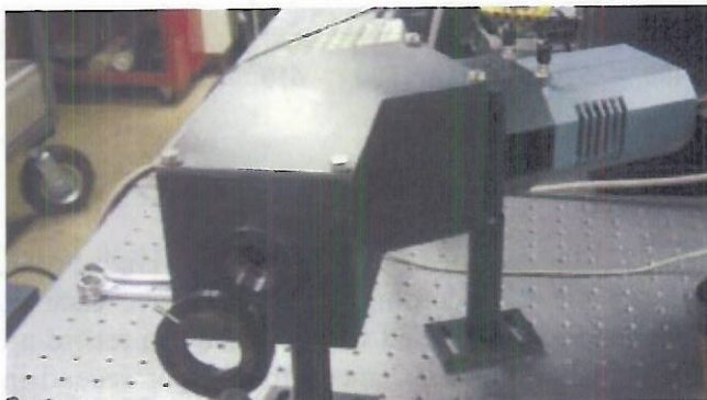
Figure V.13 Andor FK CCD detector mounted to custom spectrometer.
