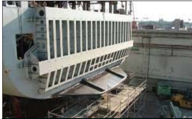
Improved Hydrodynamics Example: Stern Flaps and Hull Coatings
