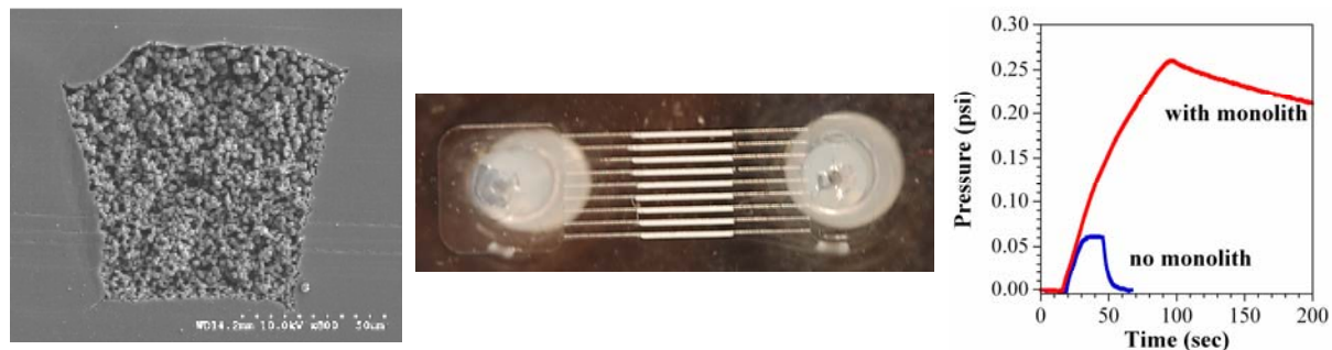
Figure 1. a) Cross-sectional SEM image of a porous polymer monolith in a PDMS microchannel. b) PPMs (white) within the channels of a nastic device. c) Pressure increase due to PPM.
