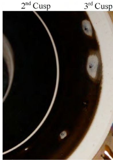
Figure 13. Photograph of 5 probes furthest downstream after recent testing. A white ring is visible in the middle is the second cusp. Large aureolas can be seen around four of the probes.
