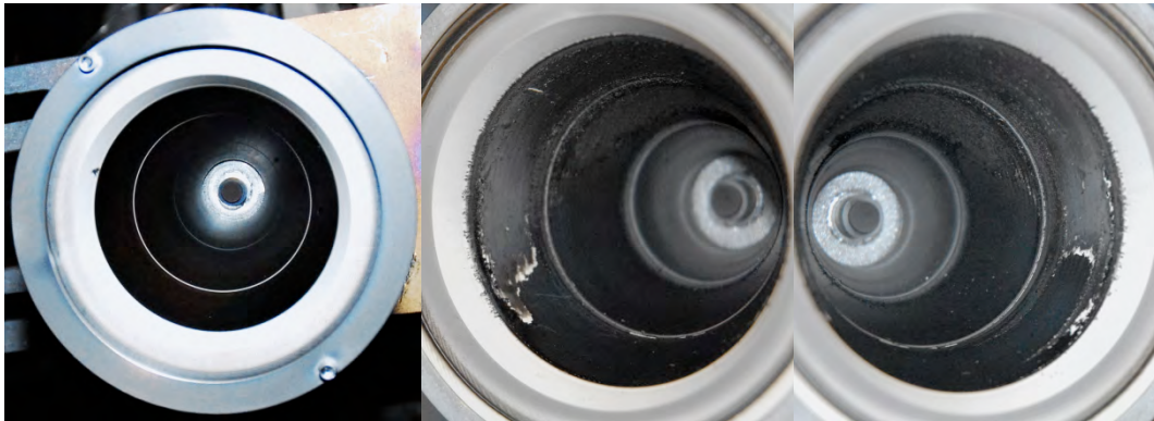
Figure 49: Left: The thruster after 65-70 h of operation, but before the start of the long duration test. The photos in the middle and on the right show the DCFT after the long test. Regions with erosion are evident as bright white rings. The uneven, but somewhat symmetrical pattern of deposition is also visible. The cathode was located above the thruster in these pictures, and to the left of the thruster in the left-hand photo.
