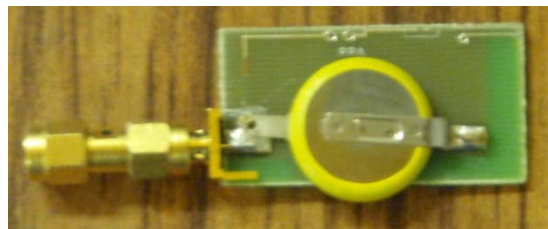
Figure 3.7: Battery attachment for the DUT
