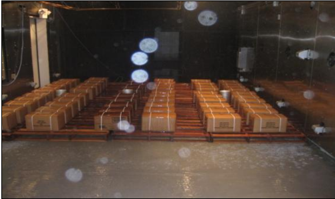
Figure 40. MRE™ test samples during 8 h high intensity rain exposure
