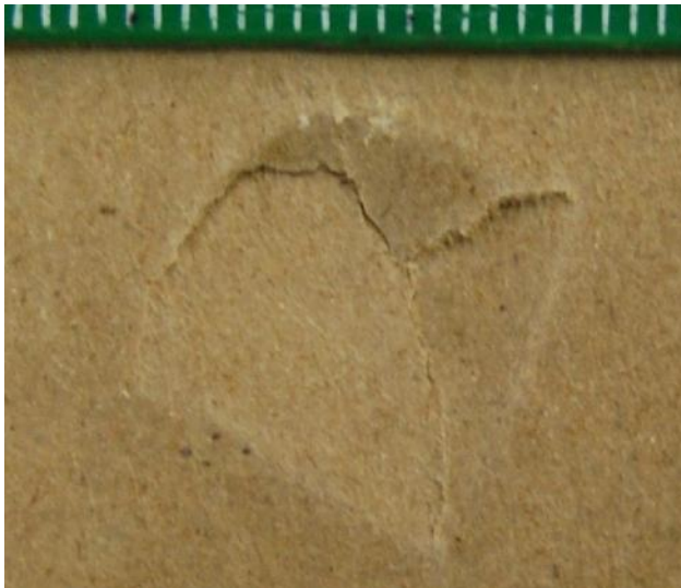
Figure 32. Fractured surface of 75Dip sample after impact test
