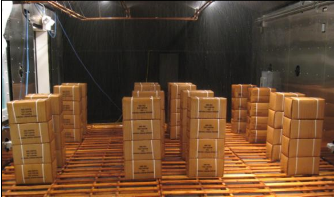
Figure 39. MRE™ test samples during 8 h stack rain test
