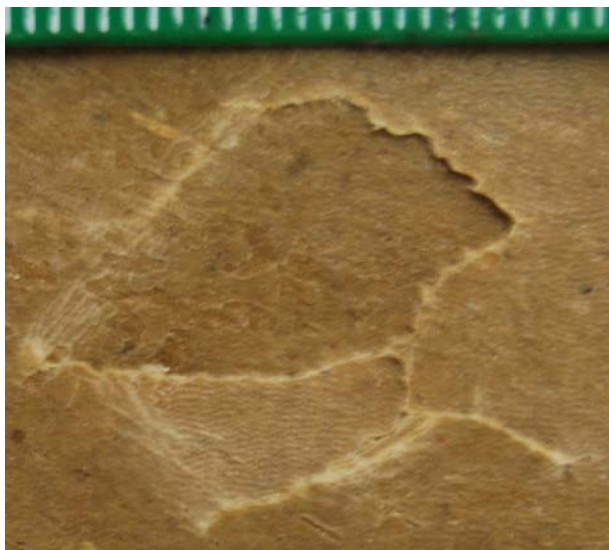
Figure 33. Fractured surface of 75Melt sample after impact test
