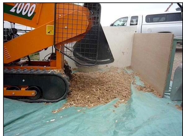
Figure A-31. Shredded fiberboard being discharged
