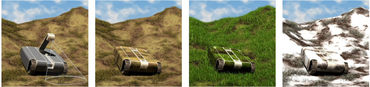
Figure 9. A virtual ISR robot using the AEC system in various simulated environments. An image is taken of the local environment (as illustrated in the left image) and supplied as the input image to the real color-texture-synthesis process to generate the camouflage pattern displayed on the exterior surface of the robot.
