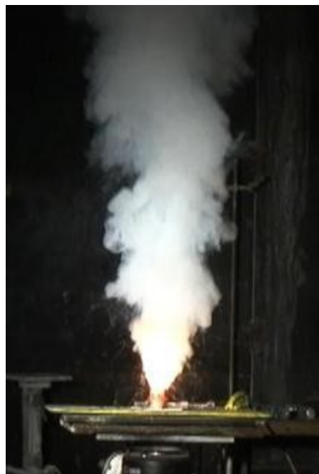
Figure 4. Test of an HHS tube containing the 2% calcium stearate composition from Table 4.
