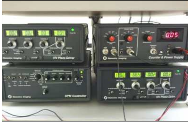
Figure 12. Upper Left Module: High Voltage Piezo Driver for the lower stage. Lower Left Module: SPM Controller. Upper Right Module: Counter and Power Supply. Lower Right Module: High Voltage Piezo Driver for the upper stage.
