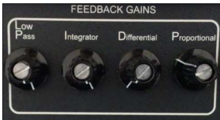
Figure 23. Typical Feedback Gain settings on the SPM Controller. The Low Pass filter and Integrator settings are rotated fully clockwise to the maximum value. The Differential setting is rotated fully counter-clockwise to the minimum value. The Proportional setting is rotated clock-wise to the "10 o'clock" position.
