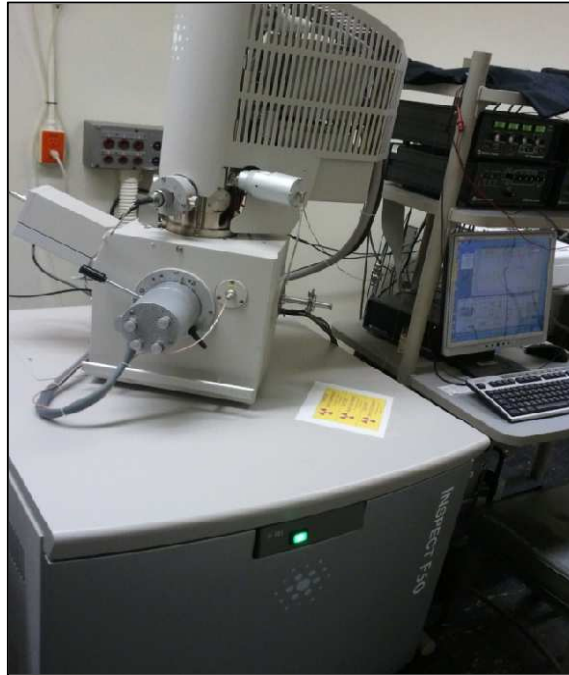
Figure 14. FEI Inspect F50 Scanning Electron Microscope. The microscope is controlled by an independent computer.
