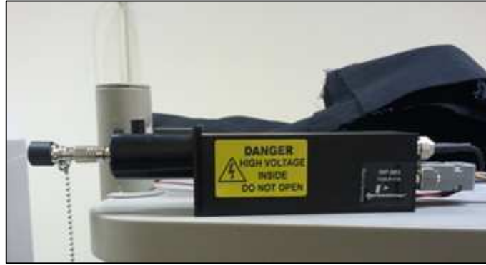
Figure 11. Photomultiplier tube fed by the fiber optic wire from the NSOM probe.
