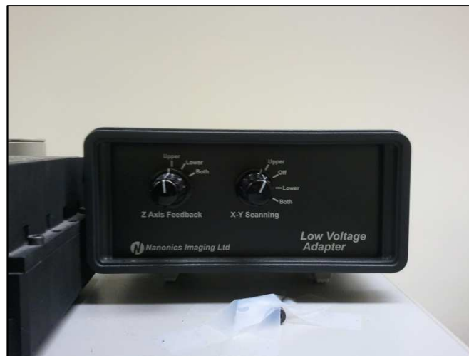
Figure 10. The Low Voltage Adapter is used to select either the upper or lower scanner for scanning and feedback adjustments.
