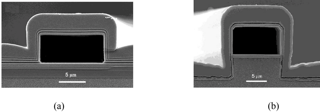
Figure 2.6 SEM pictures of ARROW: (a) Non-pretched ARROW (b) Pretched ARROW
