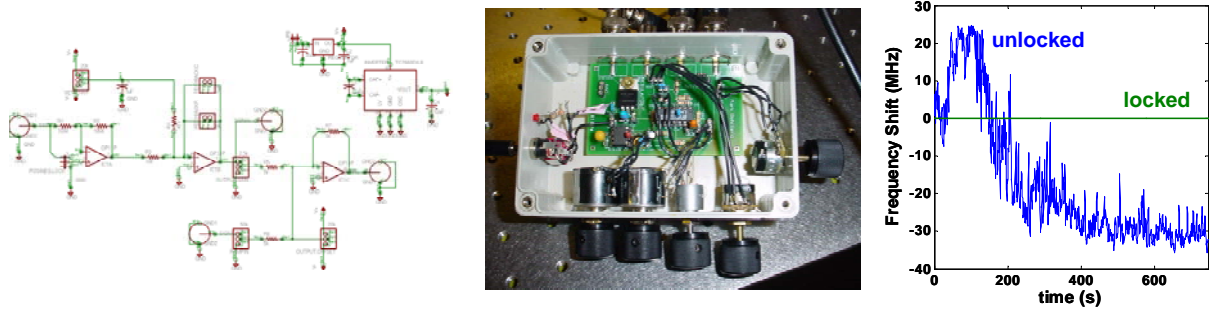
Laser frequency locking circuit, physical implementation, and performance.
