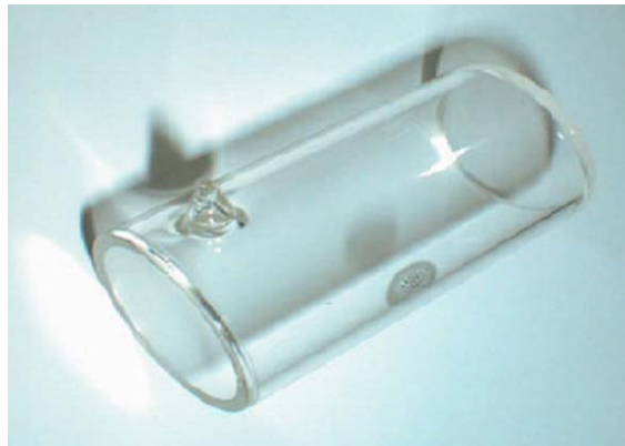
Figure 2. 8 A conventional atomic vapor cell.
