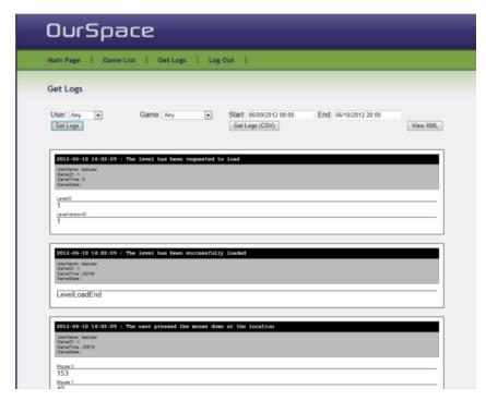
Get Logs (CSV) allows the user to retrieve the data in a CSV format
