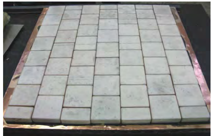
Figure 9: Images of large multi-tile array of aluminum oxide tiles actively brazed to Kovar ® /316L SS pyramidal core backing using copper and Kovar ® interlayers.
