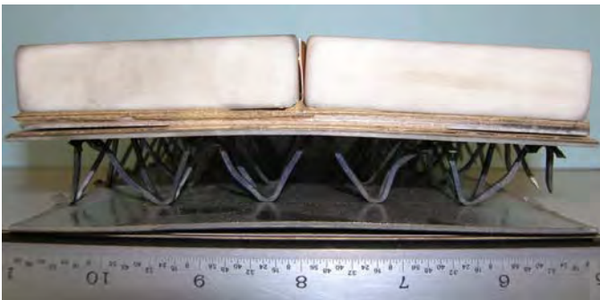
Figure 8: Unsuccessful four-tile actively brazed ceramic-metal sample with a lower core density pyramidal core backing.
