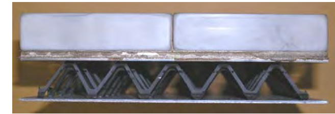
Figure 6: Example of a four-tile actively brazed ceramic-metal sample with Kovar ® /316L SS pyramidal core backing.
