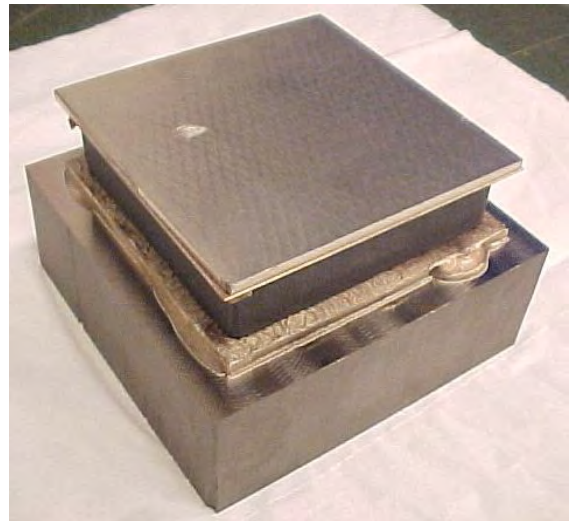
Figure 4: Example of a single tile actively brazed ceramic-metal sample with thick titanium backing.
