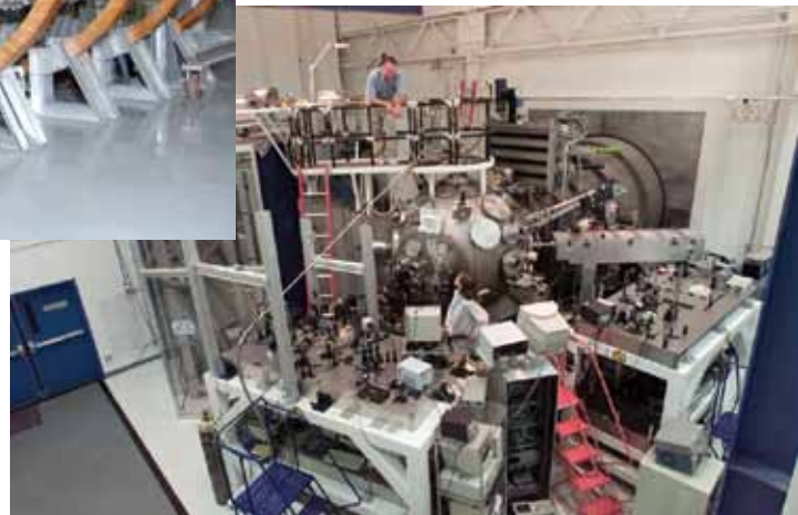
NRL's Nike target chamber, the largest krypton fluoride (KrF) laser facility in the world, where targets are accelerated to the velocities needed for fusion implosions.
