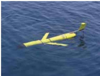
Slocum gliders, autonomous underwater vehicles, are equipped with temperature/salinity/pressure sensors and with real-time satellite connection to the Iridium network.
