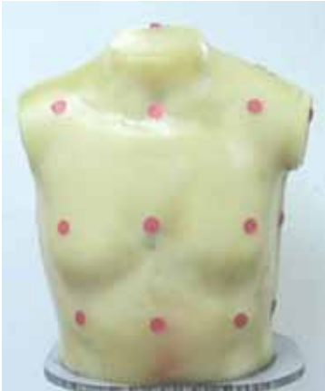
NRL GelMan human surrogate technology is used to record and analyze dynamic responses to blast pressure and impacts. GelMan torso measurement systems assess pressure transmission directly into the body, and through body armor into the body. GelMan-Brain systems quantify headborne protective equipment performance with the aim of reducing traumatic brain injury.
