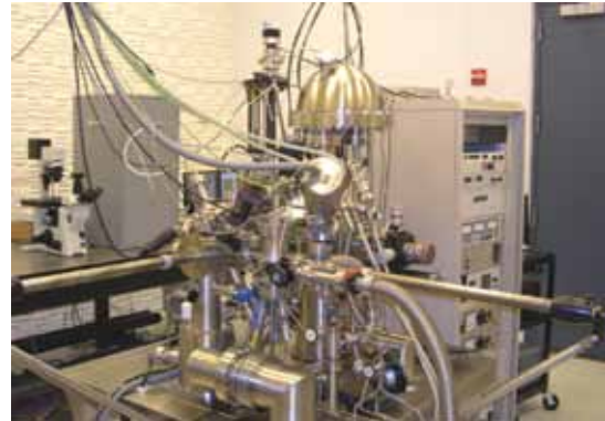
The Optical Sciences Surface Characterization Facility includes instrumentation for ultraviolet and X-ray photoemission spectroscopy (UPS and XPS), atomic force and scanning tunneling microscopy (AFM and STM), and STM-induced light emission (STM-LE) measurements.
