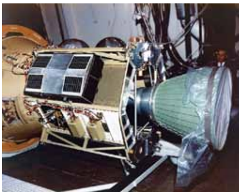
TIMATION I satellite (rectangular object) shown mounted on the side of its launch vehicle.
