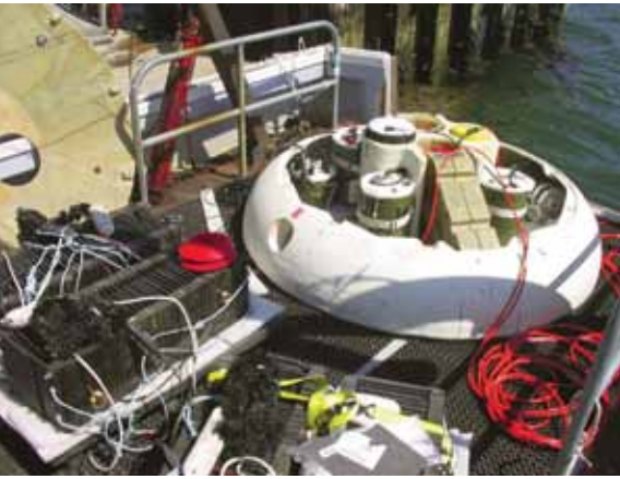
Field testing an oceanographic mooring powered by a benthic microbial fuel cell.
