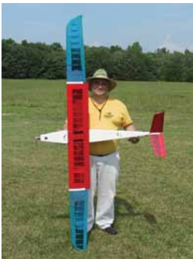
The late James Kellogg with the 6-lb Spider Lion. The Spider Lion flew for 3 hr and 19 min on 15 g of hydrogen fuel in November 2005.
