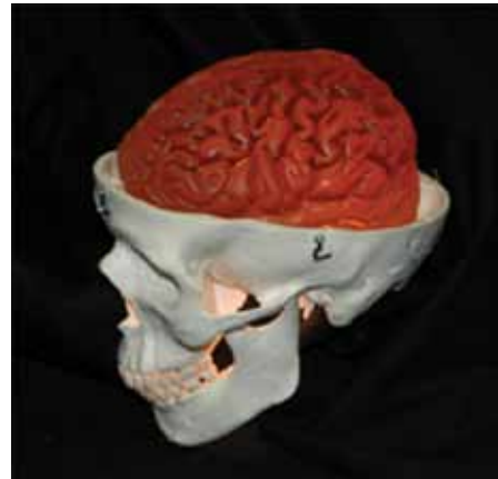
NRL GelMan human surrogate technology is used to record and analyze dynamic responses to blast pressure and impacts. GelMan torso measurement systems assess pressure transmission directly into the body, and through body armor into the body. GelMan-Brain systems quantify headborne protective equipment performance with the aim of reducing traumatic brain injury.
