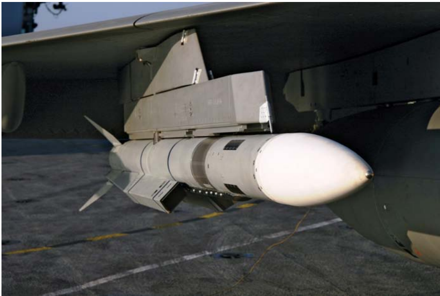
Figure 8. Technologies such as the ramjet-derivative propulsion system on the MDNA Meteor are beginning to enable high-speed AAMs with greater range and terminal maneuverability. (Courtesy MBDA–Th Wurtz.)
