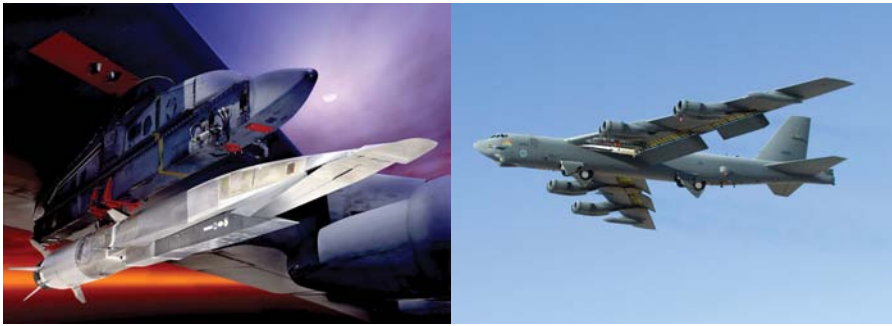
Figure 30. Advances made over the past decade in scramjet propulsion technologies embodied in the X-51 demonstrator can allow development of high-speed cruise missiles and other capabilities to support long-range strike on critical targets in A2/AD environments. (Courtesy US Air Force.)
