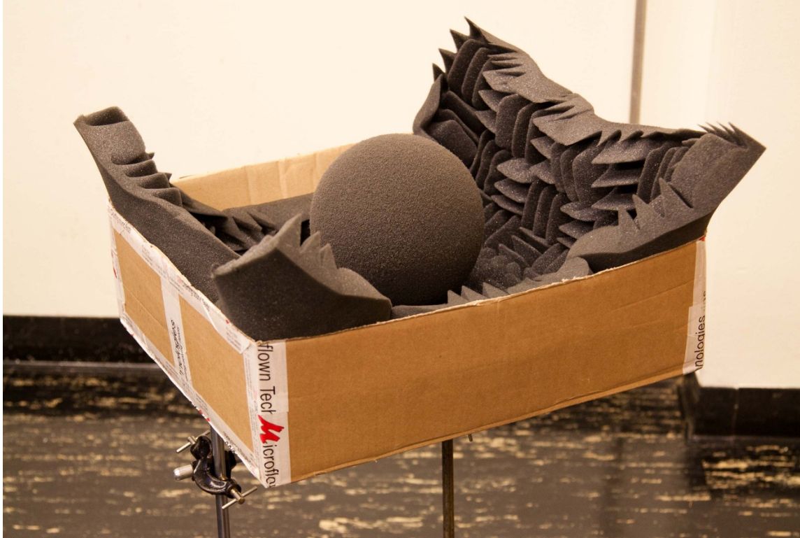
Figure 17. Revised setup of single Microflown USP and anti-reflection foam box still need picture
