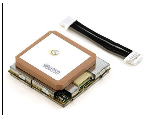
Figure 5. EM-406A OEM GPS unit (From [12]).
