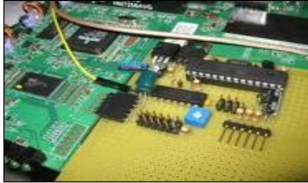
Figure 2. MAX232 and components (From [11]).
