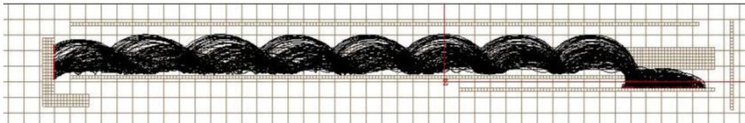
**Figure. 7. SIMION simulation of the injected beam configuration of the CFA with the beam injection at right and the collector at left.**
