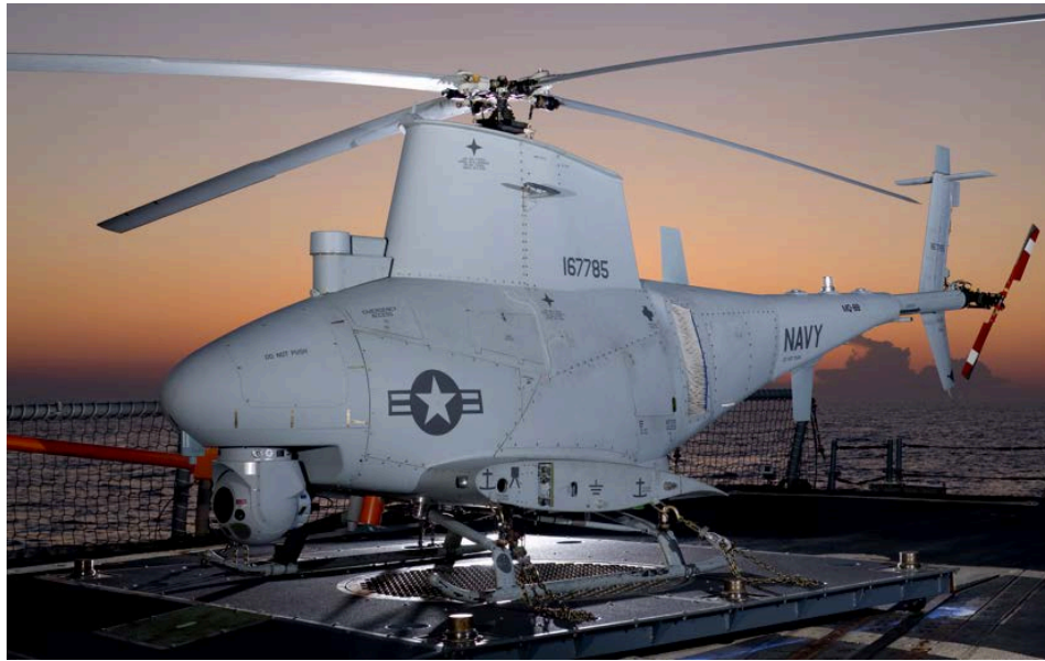
Figure 6. Fire Scout VTUAV landing aboard USS McInerney (From Northrop Grumman Corporation) 37
