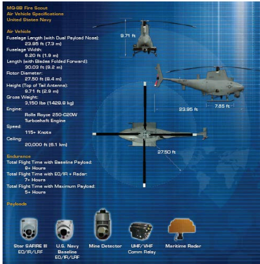
Figure 5. Fire Scout VTUAV Specifications (From Northrop Grumman Corporation) 27
