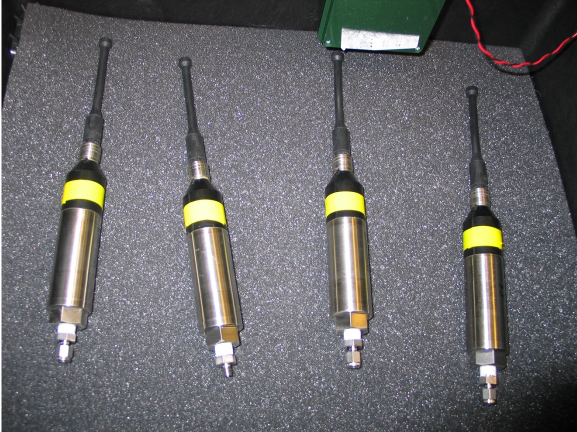
Diver-worn Depth Sensor (DWDS) — the Honeywell Model PPTR0300AP5VB Precision Pressure Transducer (PPT) — selected for the DWDS. These pressure sensors are shown with molded submersible waterproof 6-pin male connectors and ¼" NPT pressure ports. SUBCONN submersible MCIL6F and MCIL6M connectors are used to attach the depth sensor to the cable.
