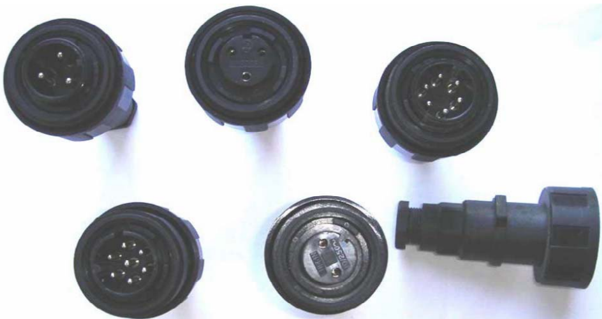
BULGIN Circular Connector, Buccaneer Series, IP68-rated. Various connectors were selected that would not allow cross connection of sources, three contacts for AC power, two contacts for DC power, six contacts for data, and so forth.
