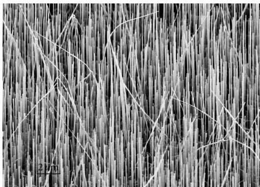
FIGURE 3: A typical SEM image of the nanowires growth with some extremely long nanowires.
