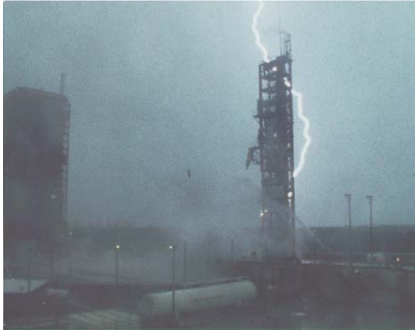
Figure 2. Triggered lightning strike to AC-67 in 1987. Only seconds after liftoff, the lightning followed the exhaust plume to the ground. (From: Roeder and McNamara 2006)
