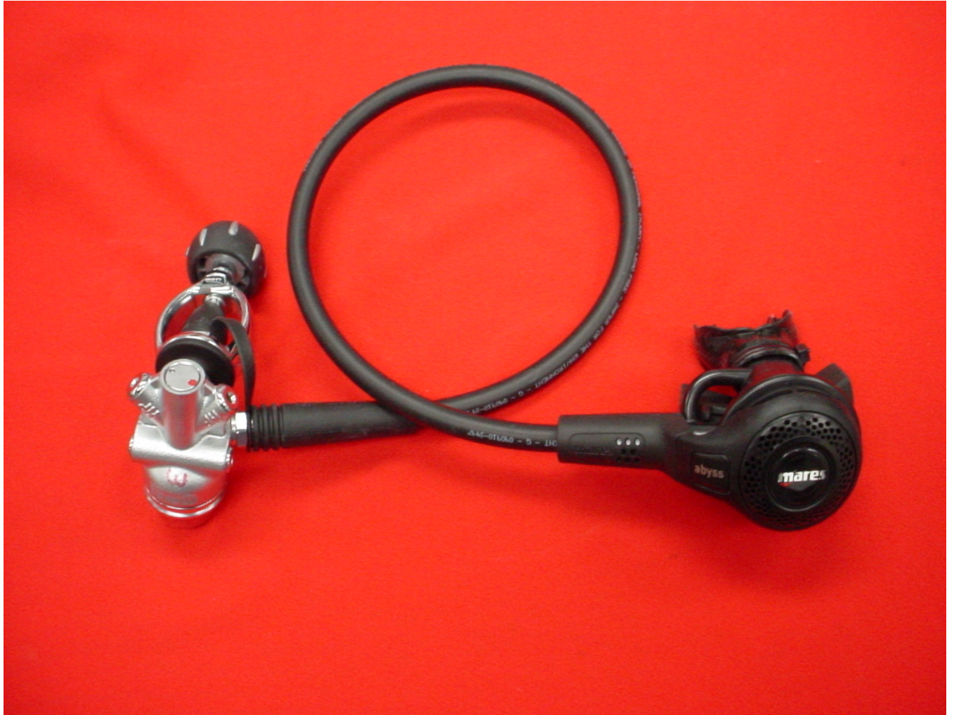
Figure 1. Tested Mares Abyss 22 Navy regulator, with first-stage assembly (left, with dust cap in place), rubber-jacketed intermediate pressure hose (middle), and second-stage assembly (right).
