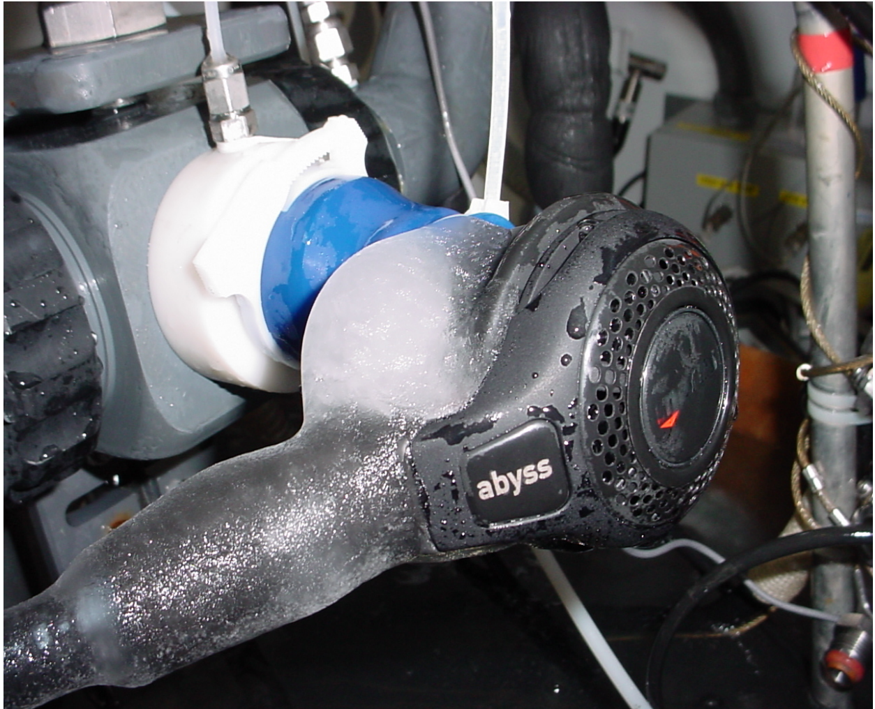
Figure 8. Typical second-stage assembly of the Mares Abyss 22 Navy regulator, with external icing after a Phase 2 exposure. The regulator is shown above the water. Note the blue mouthpiece adaptor, white oral static pressure pick-up ring, and gray routing block attached for testing.
