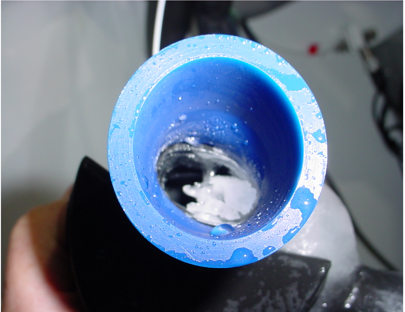
Figure 9. Typical second-stage assembly of the Mares Abyss 22 Navy regulator, with internal icing after a Phase 2 exposure. The regulator is shown above the water. Note the blue mouthpiece adaptor (foreground) installed for testing.
