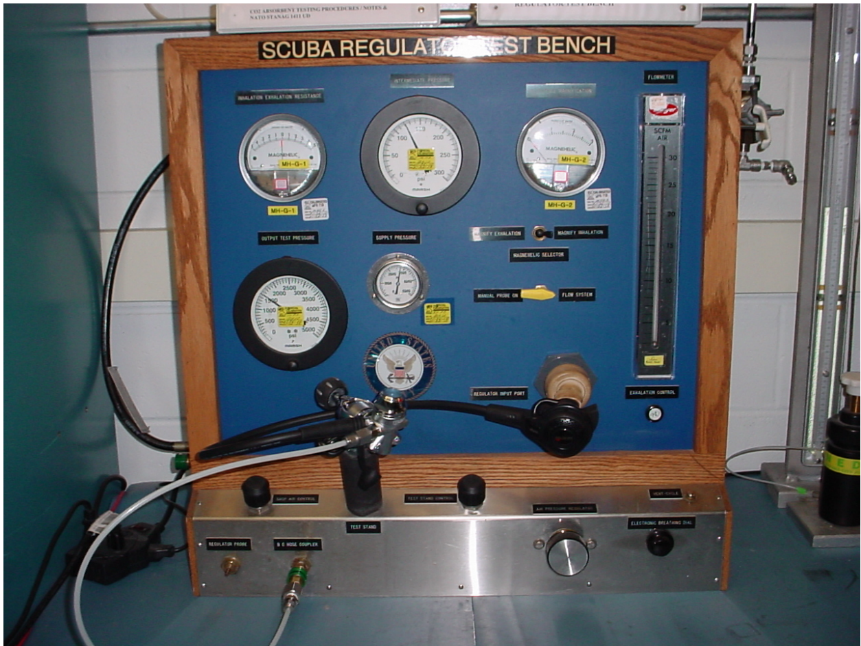
Figure 6. Typical Mares Abyss 22 Navy regulator, attached to the dry bench apparatus for Phase 1 testing.
