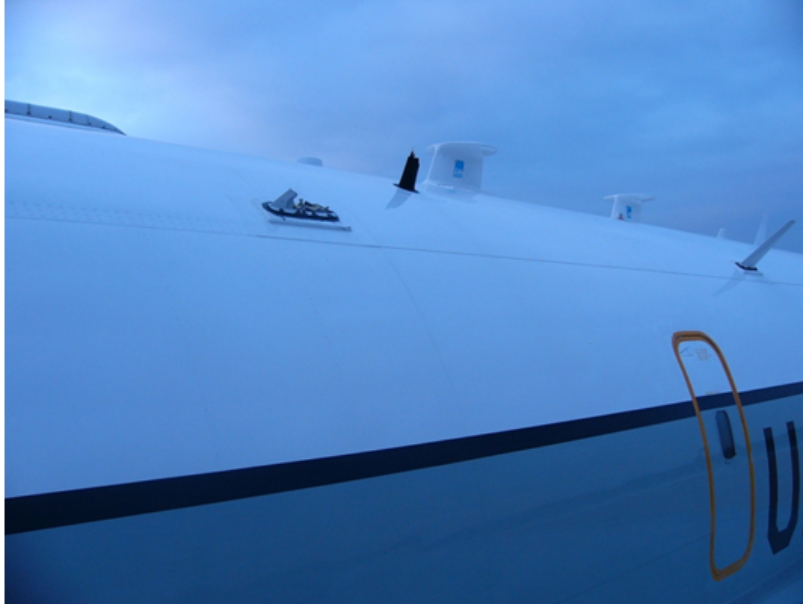
Figure 1.5: Damage to UHF3 and HF long-wire mast from the November 2009 incident [3]
