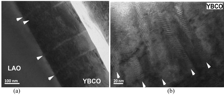
FIGURE 4. Cross-sectional TEM micrographs of YBCO+BGEO samples showing the nanocolumns at two different magnifications a) Low magnification b) High magnification
