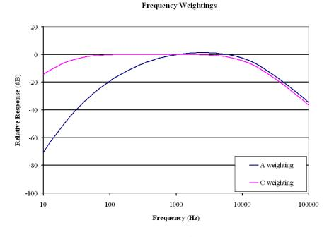
Source: Peterson and Gross (1974). Figure A1. A- and C-frequency weighting characteristics.
