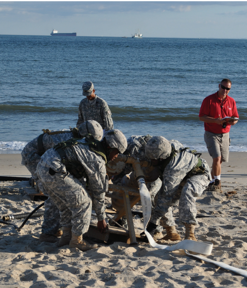
Soldiers from the 610th Quartermaster Company, Saint Thomas, U.S. Virgin Islands, deploy the cyclone separator for a 3,000-gallon-per-hour ROWPU as part of the ROWPU RODEO competition at Fort Story, Virginia. (Photo by SGT Paul Kindzierski, 262d Quartermaster Battalion)
