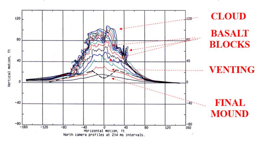
VENTING BEGAN ~ 400 MS WITH INDIVIDUAL BASALT BLOCKS EMERGING IN NEAR VERTICAL TRAJECTORIES, BY 1 SEC BASALT BLOCKS WERE BYPASSING DUST, BY 2 1/2 SEC THEY WERE FALLING WHILE DUST CONTINUED TO RISE FORMING THE CLOUD, LAST FRAME ANALYZED @ 2.782 SEC
