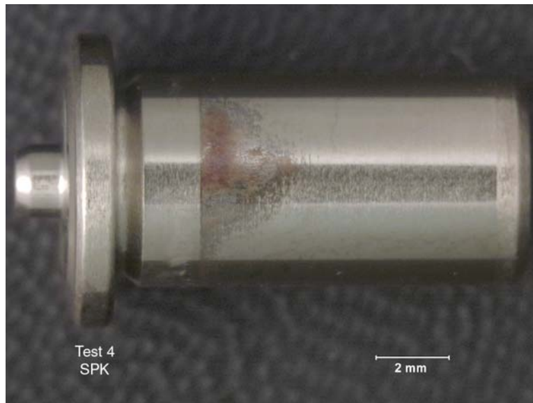
Figure 29 - AF7868 SPK, Upper Hydraulic Coupler Piston, Profile
