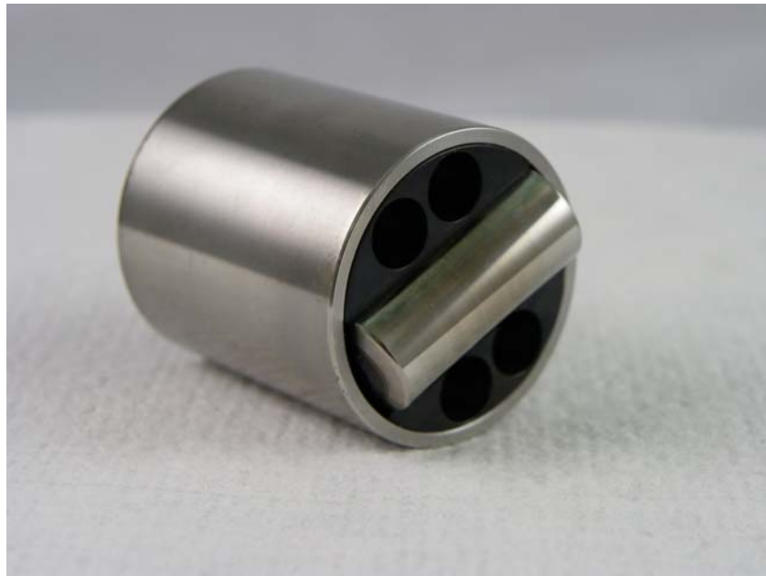
Figure 19 - AF7469 ULSD, Right Cam Follower Roller
