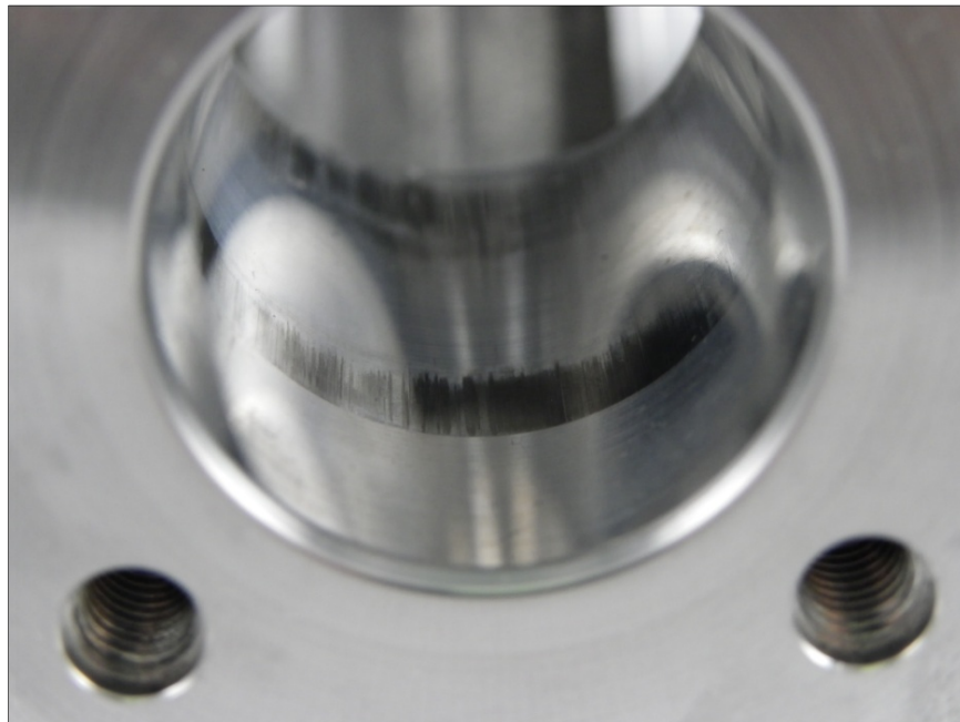
Figure 26 – Post-Test SPK Pump Body Bore Polish (Light Scuffing)
