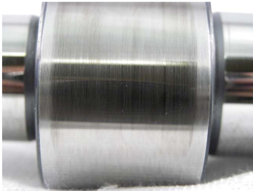
Figure 16 - AF7868 SPK, HPCR Pump Camshaft, Lobe Surface Close-up
