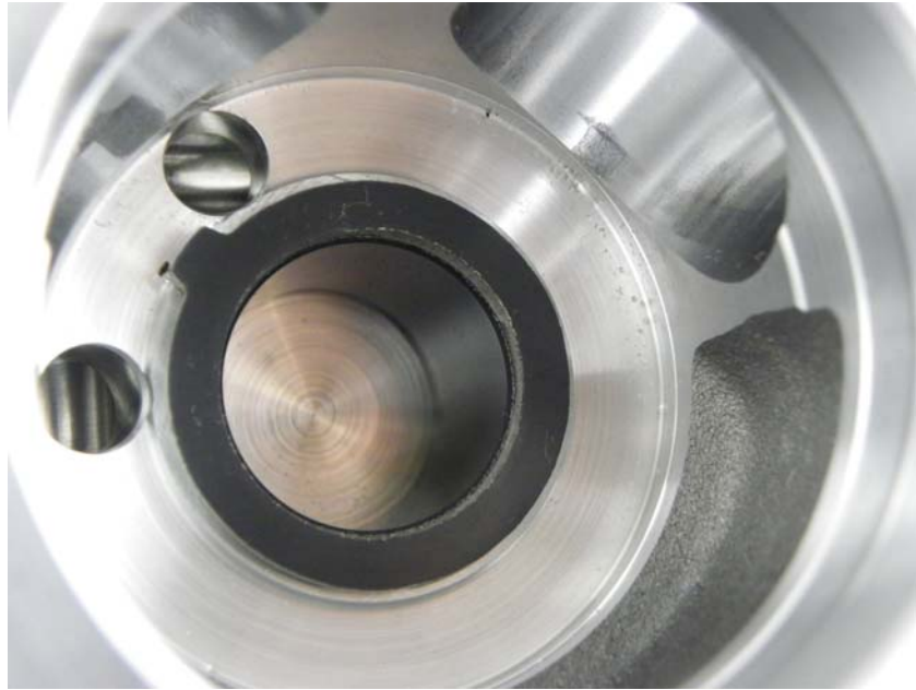
Figure 13 - AF7801 JP8, Rear Pump Body Camshaft Bushing
