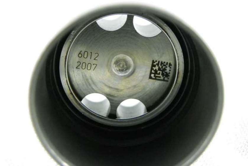
Figure 26 - AF7824 50/50 JP8/SPK, Right Cam Follower Undercrown
