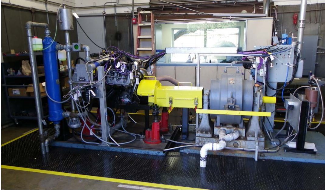
Figure 1 - Ford 6.7L Test Engine Installation
