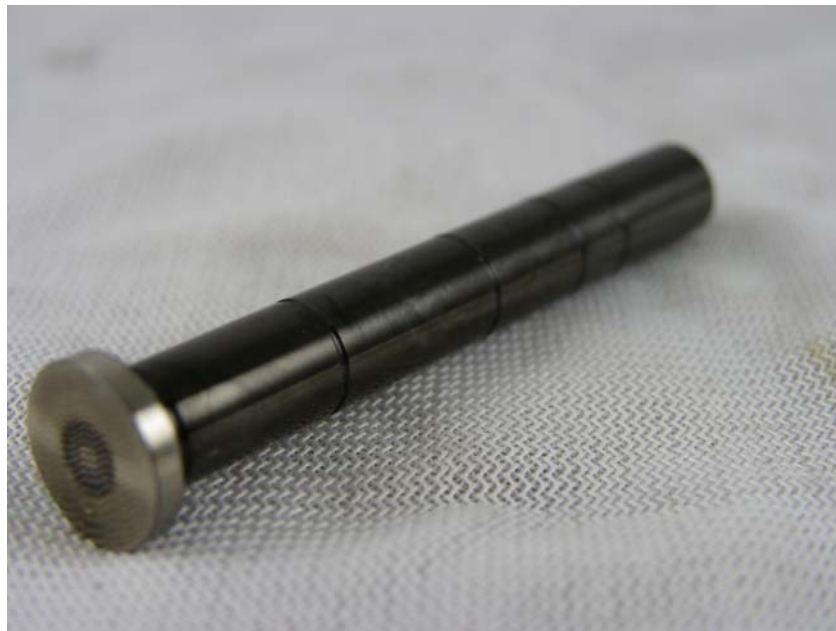
Figure 20 - AF7801 JP8, Left High Pressure Piston
