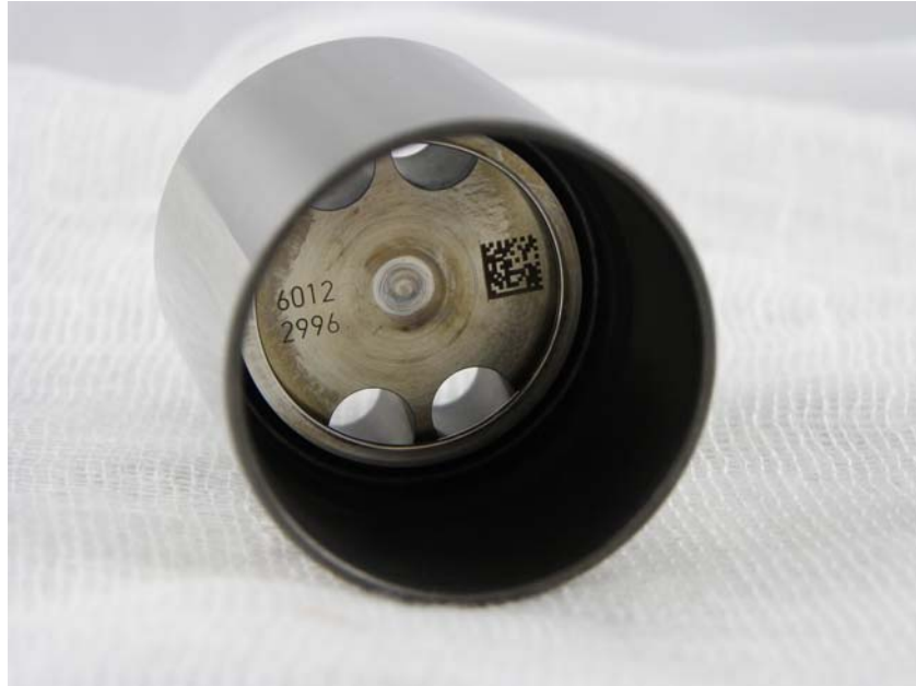
Figure 23 - AF7868 SPK, Right Cam Follower Undercrown
