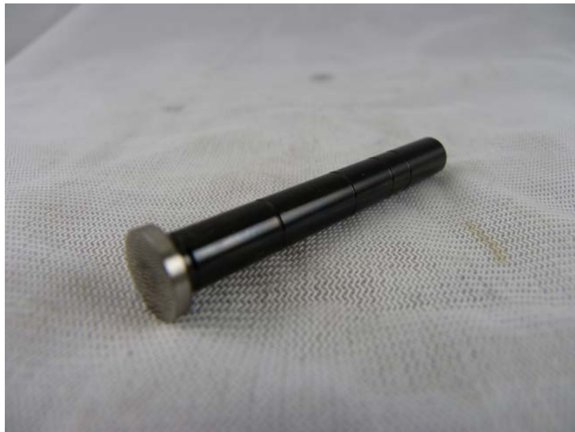
Figure 17 - AF7469 ULSD, Left High Pressure Plunger
