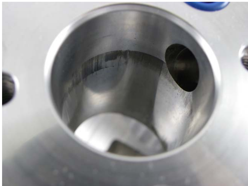
Figure 10 - AF7824 50/50 JP8/SPK, Post Test, Left Pump Bore Close
