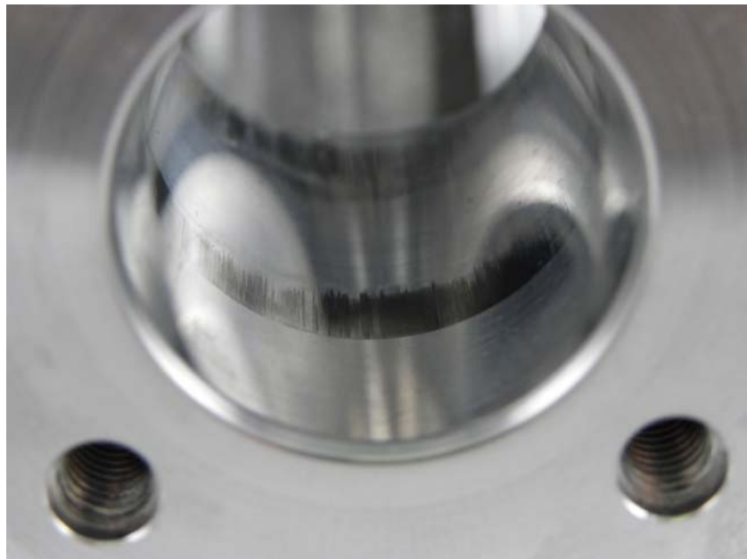
Figure 12 - AF7868 SPK, Post Test, Right Pump Bore Close
