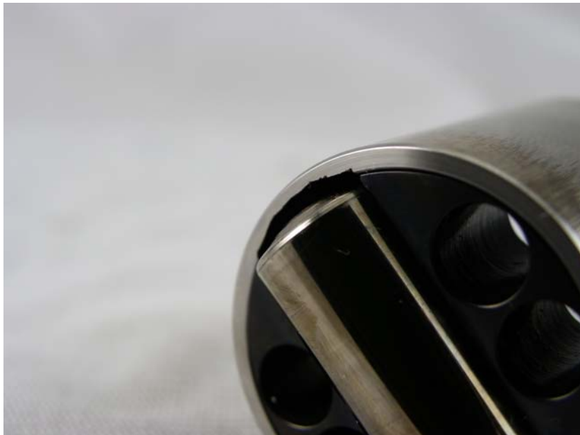
Figure 20 - AF7824 50/50 JP8/SPK, Left Hand Follower Roller Wear - 2
