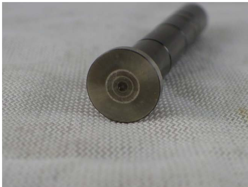
Figure 23 - AF7824 50/50 JP8/SPK, Left High Pressure Piston
