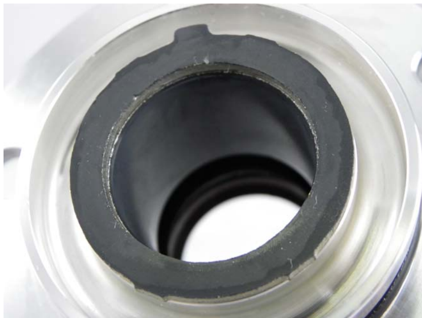
Figure 14 - AF7824 50/50 JP8/SPK, Front Pump Body Camshaft Bushing
