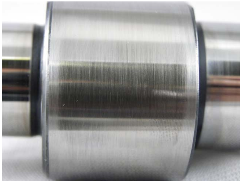
Figure 16 - AF7801 JP8, HPCR Pump Camshaft, Lobe Surface Close-up
