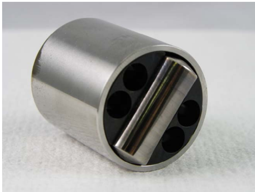
Figure 15 - AF7469 ULSD, Left Cam Follower Roller
