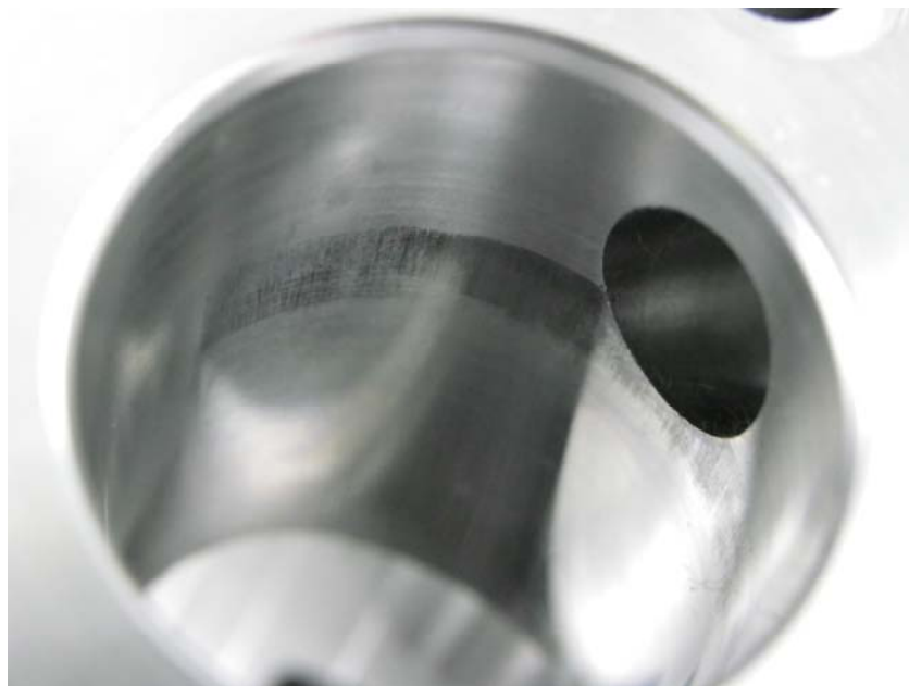
Figure 7 - AF7469 ULSD, Post Test, Left Pump Bore Close
