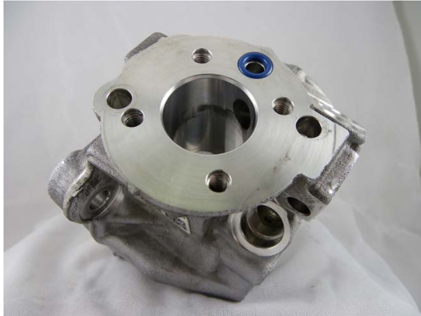
Figure 9 - AF7824 50/50 JP8/SPK, Post Test, Left Pump Bore
