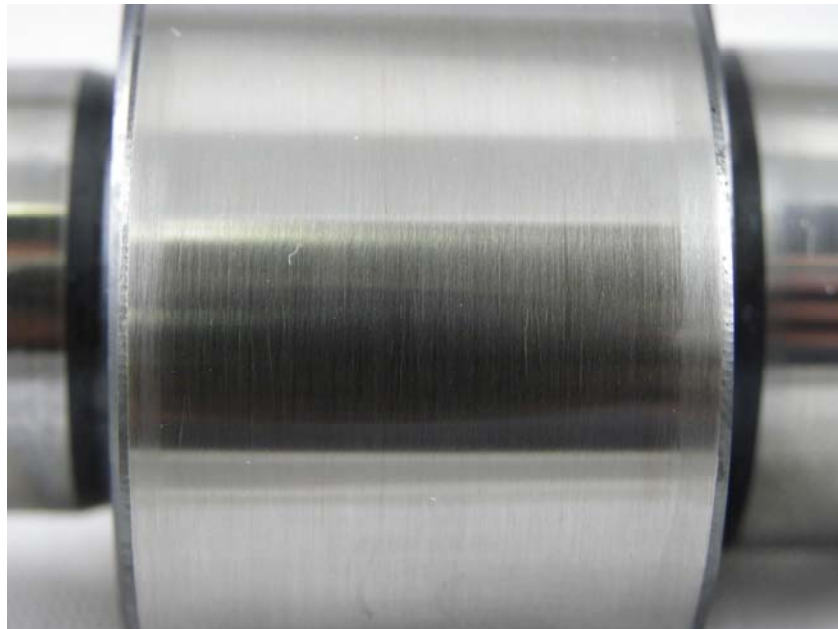
Figure 13 - AF7469 ULSD, HPCR Pump Camshaft, Lobe Surface Close-up
