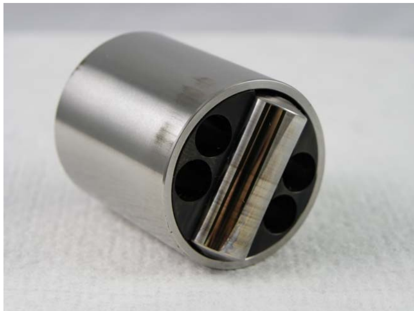
Figure 22 - AF7801 JP8, Right Cam Follower Roller
