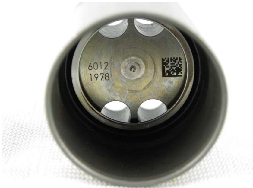
Figure 22 - AF7824 50/50 JP8/SPK, Left Cam Follower Undercrown
