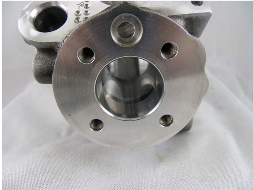
Figure 11 - AF7801 JP8, Post Test, Right Pump Bore
