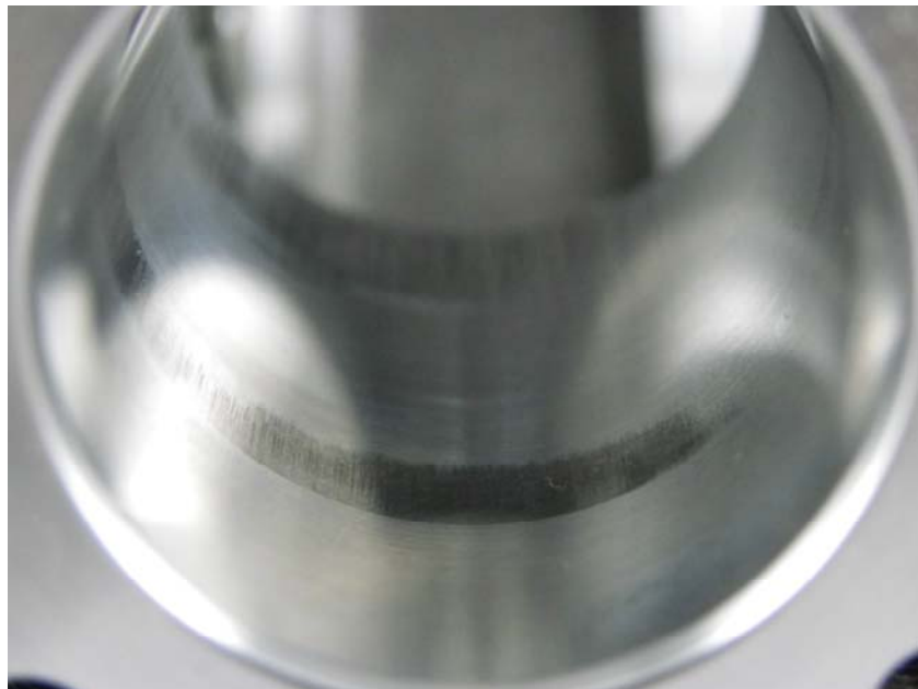
Figure 9 - AF7469 ULSD, Post Test, Right Pump Bore Close
