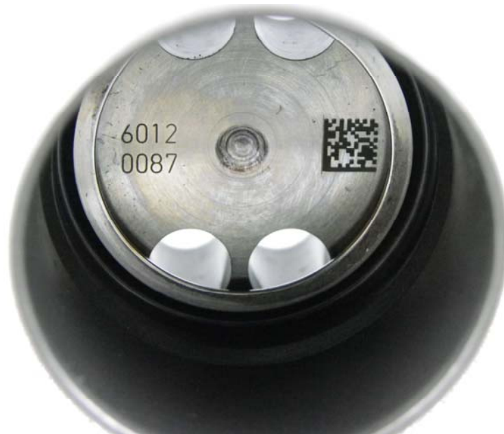
Figure 23 - AF7801 JP8, Right Cam Follower Undercrown
