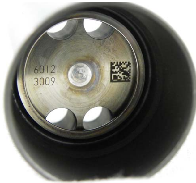
Figure 19 - AF7868 SPK, Left Cam Follower Undercrown
