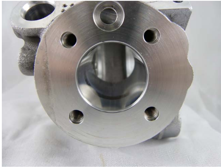
Figure 8 - AF7469 ULSD, Post Test, Right Pump Bore
