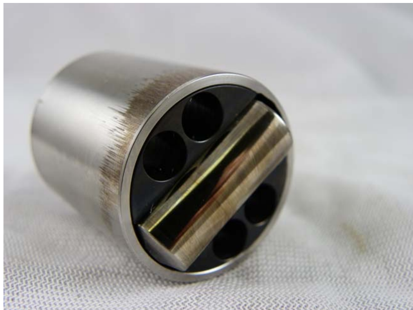
Figure 18 - AF7824 50/50 JP8/SPK, Left Cam Follower Roller
