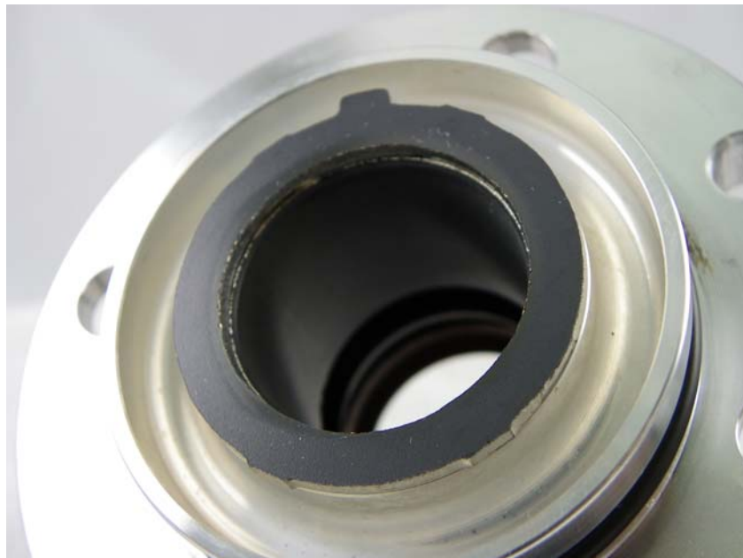
Figure 14 - AF7868 SPK, Front Pump Body Camshaft Bushing
