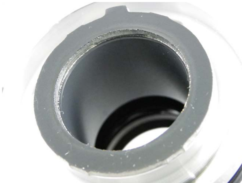
Figure 14 - AF7801 JP8, Front Pump Body Camshaft Bushing
