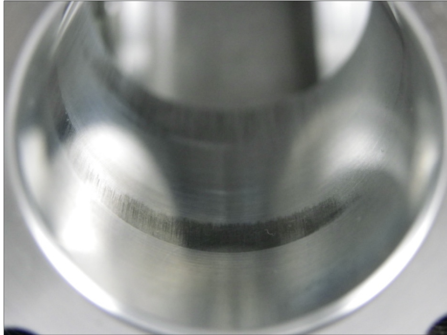
Figure 25 – Post-Test ULSD Pump Body Bore Polish
