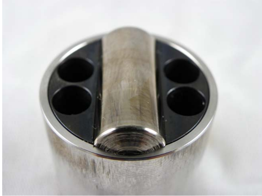
Figure 21 - AF7824 50/50 JP8/SPK, Left Hand Follower Roller Wear - 3
