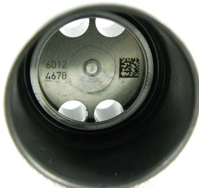
Figure 16 - AF7469 ULSD, Left Cam Follower Undercrown
