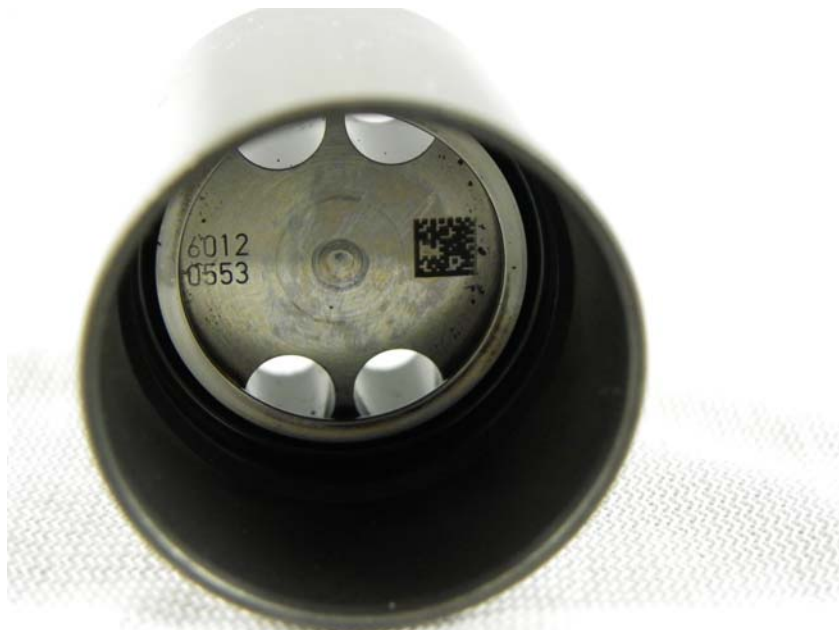
Figure 20 - AF7469 ULSD, Right Cam Follower Undercrown
