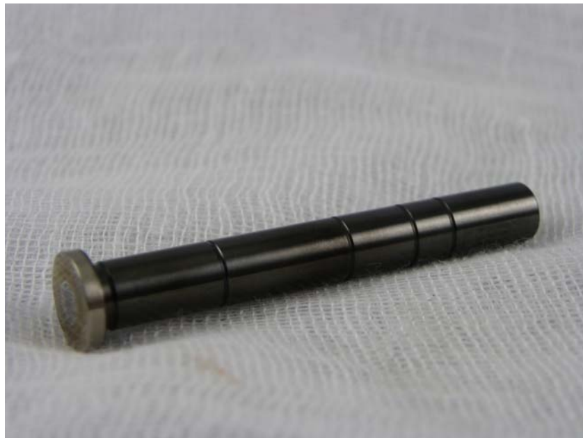
Figure 20 - AF7868 SPK, Left High Pressure Piston
