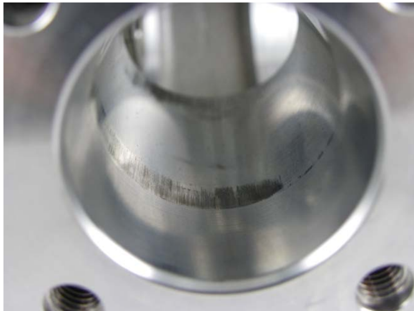
Figure 12 - AF7824 50/50 JP8/SPK, Post Test, Right Pump Bore Close
