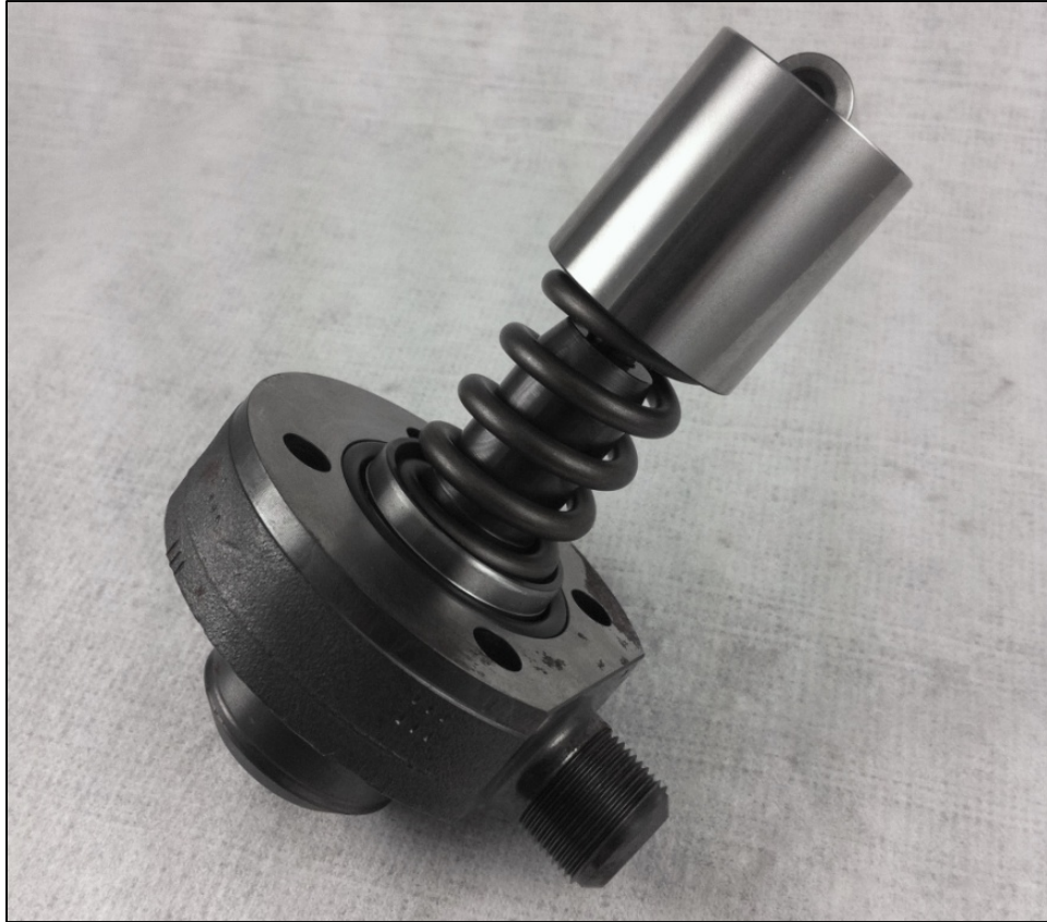
Figure 3 - Camshaft Follower & High Pressure Plunger & Barrel Assembly
