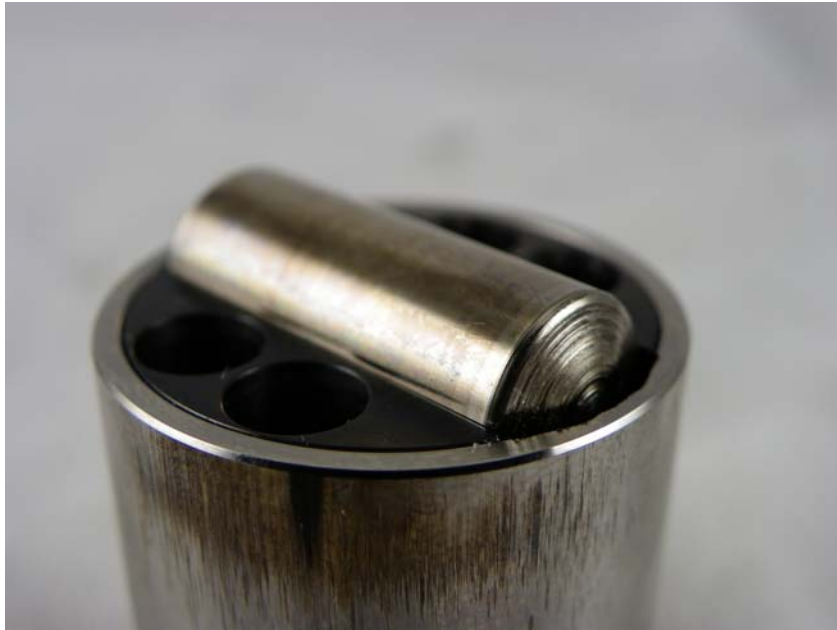
Figure 19 - AF7824 50/50 JP8/SPK, Left Hand Follower Roller Wear - 1
