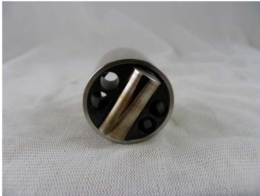
Figure 25 - AF7824 50/50 JP8/SPK, Right Cam Follower Roller
