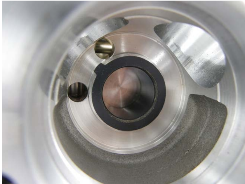
Figure 13 - AF7824 50/50 JP8/SPK, Rear Pump Body Camshaft Bushing
