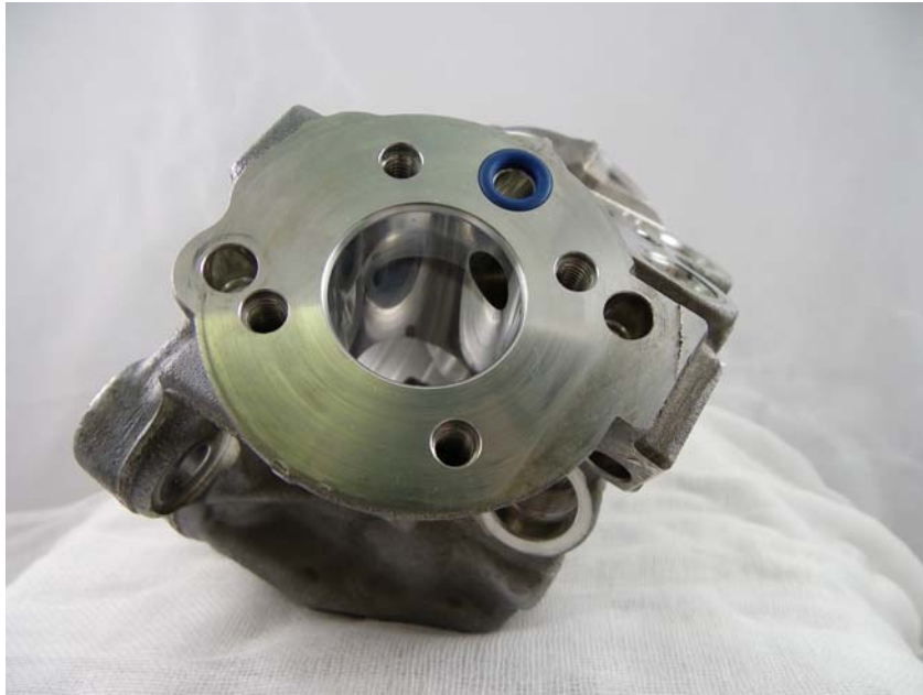
Figure 9 - AF7868 SPK, Post Test, Left Pump Bore
