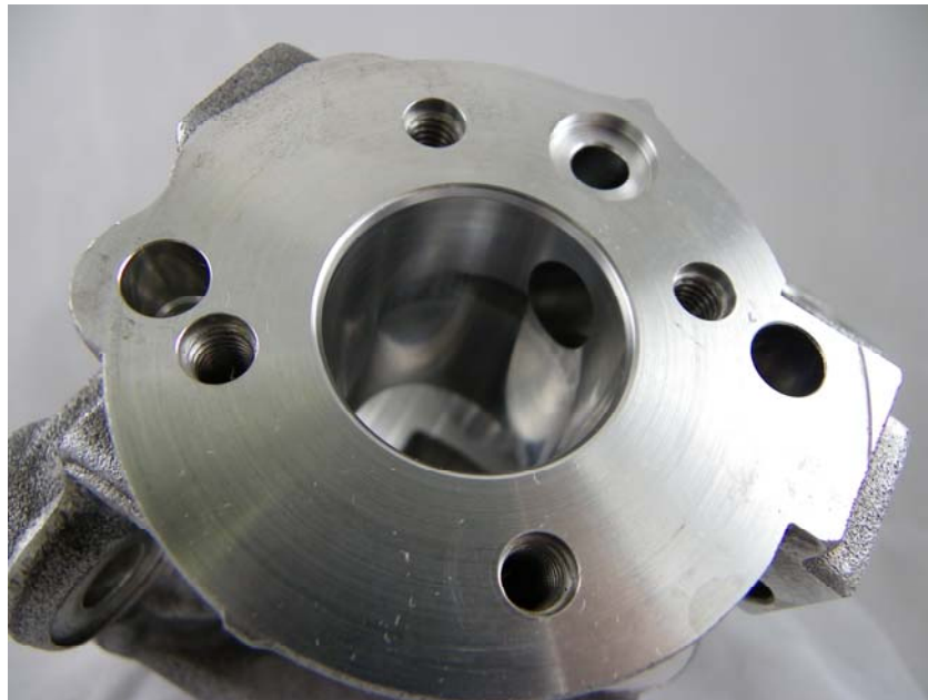
Figure 6 - AF749 ULSD, Post Test, Left Pump Bore
