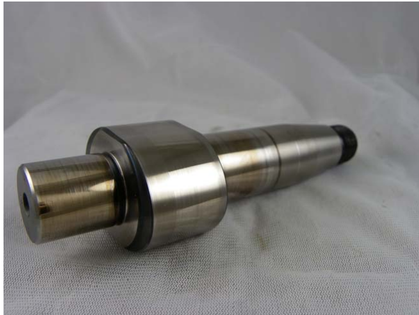
Figure 15 - AF7824 50/50 JP8/SPK, HPCR Pump Camshaft
