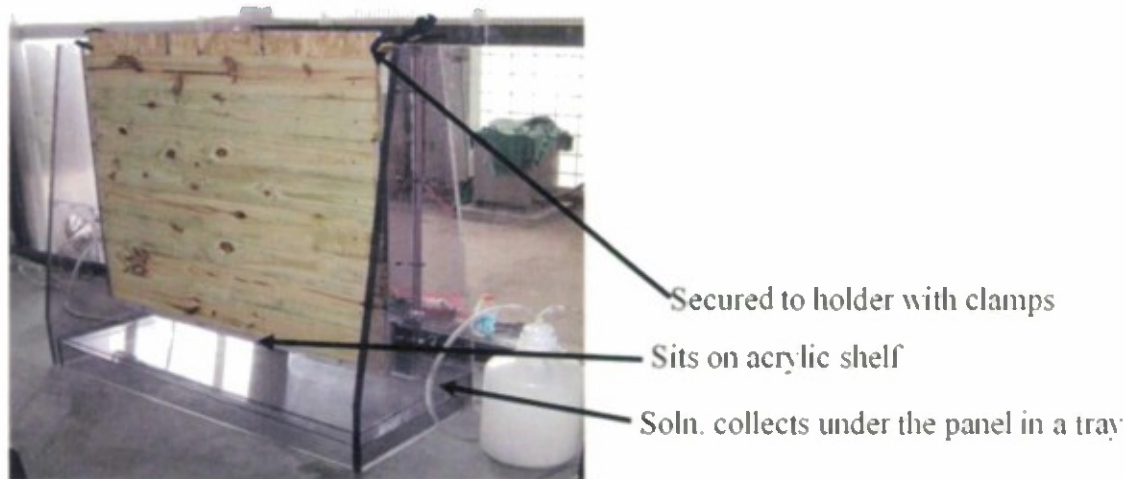
Figure 1. Panel holder for decontamination application.
