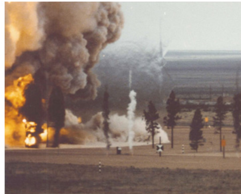
c. Measurement of airblast propagation for a large-scale HE surface burst.
