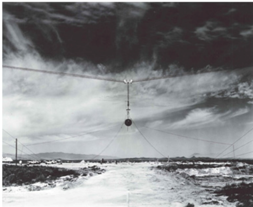
a. Photograph of a spherical explosive charge simulating nuclear airblast from an above-ground burst (1990s).
