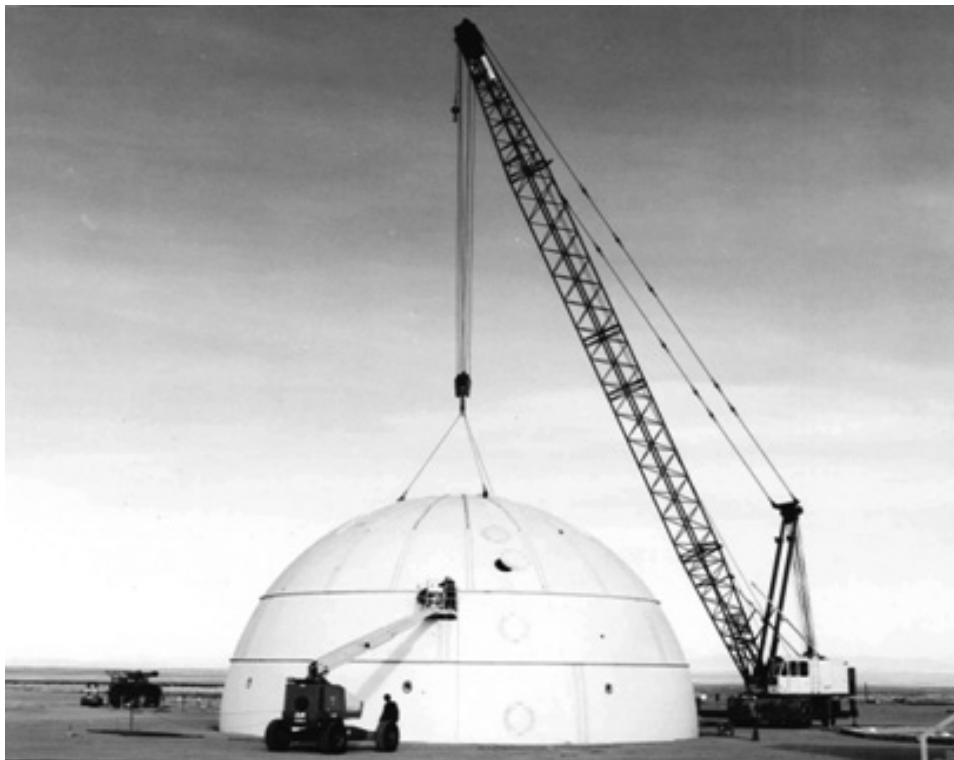
Figure 5. Photo of a hemispherical explosive charge for a large scale test simulating nuclear airblast from a surface burst (1980-1990s).
