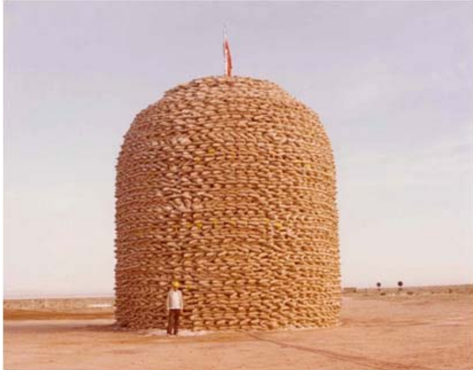
Figure 4. Photograph of a stacked explosive charge for a large scale test simulating nuclear airblast from a surface burst (1970s).
