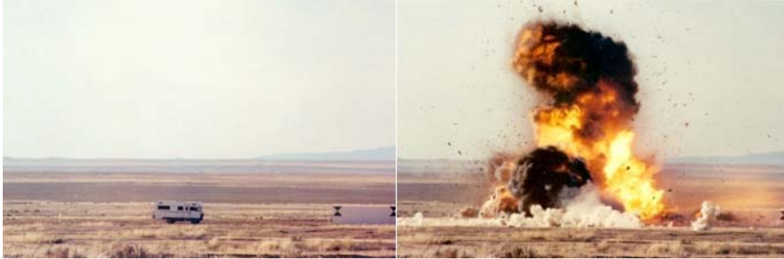
Figure 8. Vehicle bomb test conducted as part of the Anti-Terrorism testing effort.
