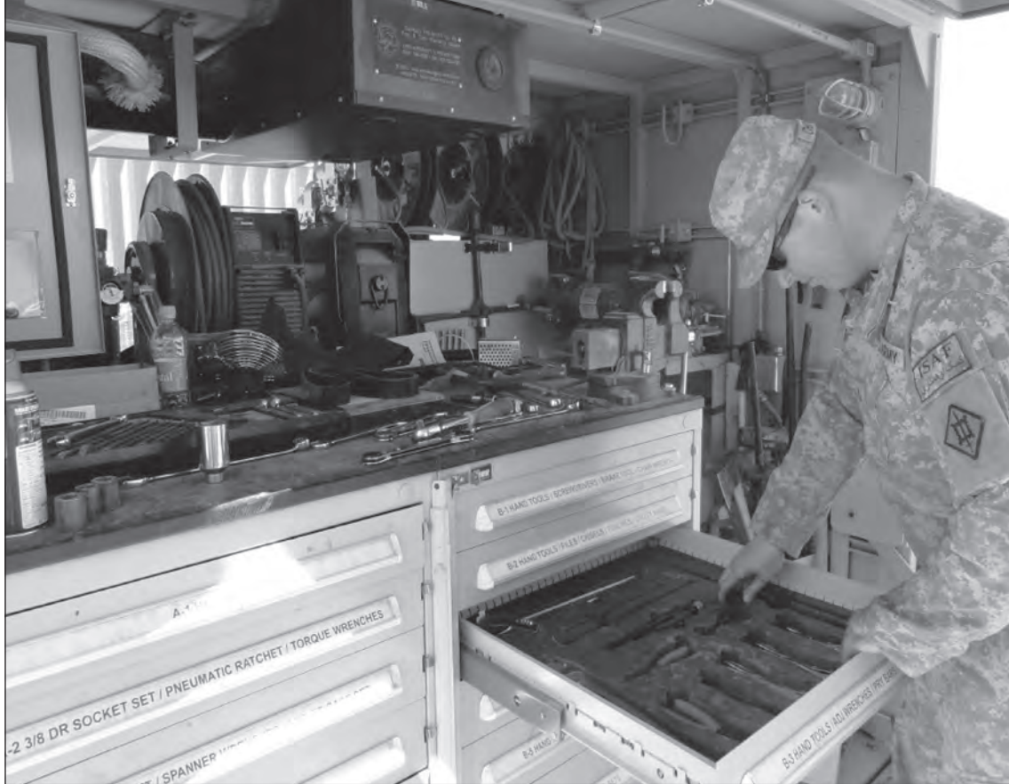
A company field maintenance team mechanic uses the Forward Repair System.
