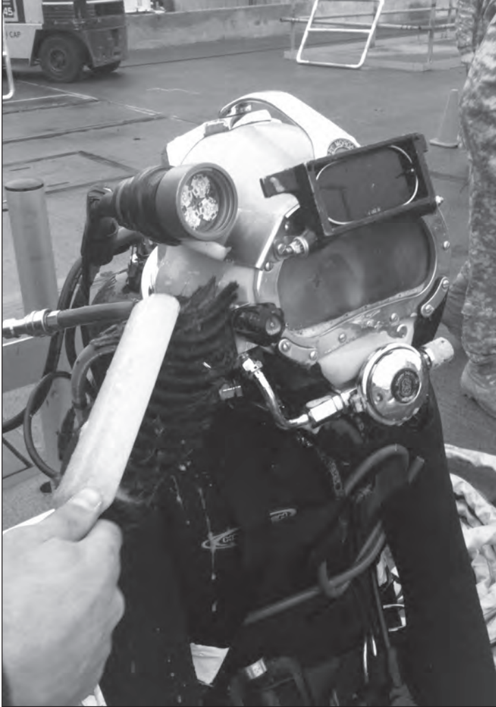
Soapy water is applied to helmet and hose connections to check for leaks.
