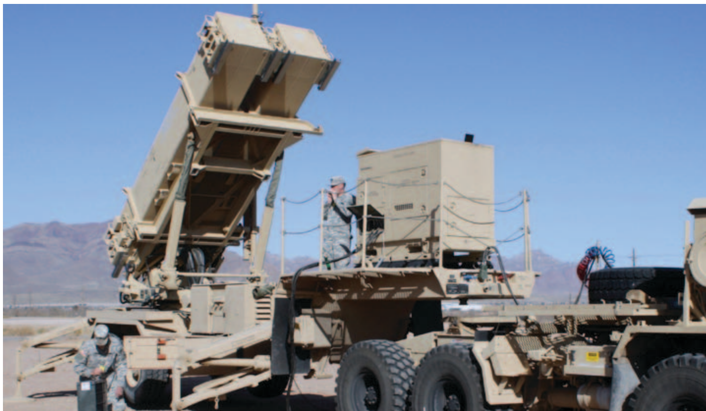
SPC Brian Deaton and PFC Edward Nedweski, power generation equipment repairers with 5th Battalion, 52nd Air Defense Artillery, perform a load bank test of a Patriot Launching Station generator during a week-long maintenance program. (Photo by CPT Dan Moore, U.S. Army)
