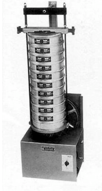
Figure 10. Sieves and shaker being used to determine grain size distributions. A Humboldt H4325 sieve shaker was used to determine grain size distributions (see LABEQUIP LTD. Available online. URL: www.labequip.com , Accessed on April 23, 2009).
