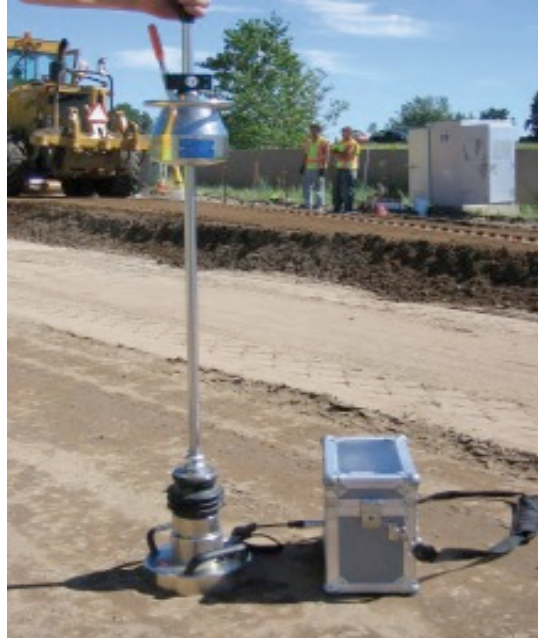
Figure 5. Light Weight Deflectometer being used to determine dynamic modulus. See David J. White, 2007. Field Validation of Intelligent Compaction Monitoring Technology for Unbound Materials. Partnership for Geotechnical Advancement, Available online. URL: ( http://www.ctre.iastate.edu/pubs/t2summaries/intel_compaction.pdf . Accessed on April 23, 2009).
