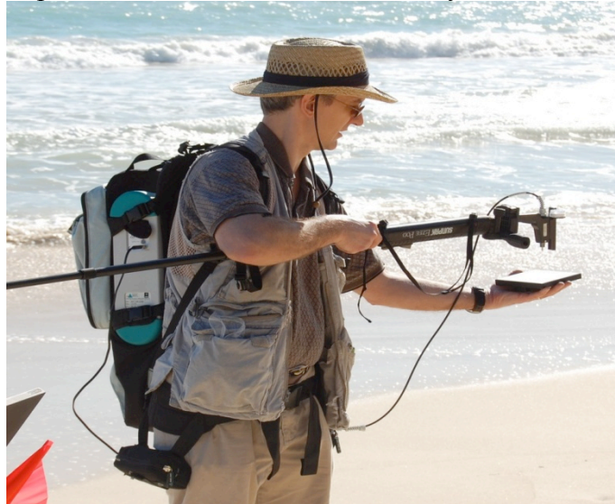
Figure 4. FieldSpec@3 Spectroradiometer. Portable spectrometers are used to collect spectra (see ASD INC., Available online. URL: http://www.asdi.com/products-fs3.asp , Accessed on April 23, 2009).
