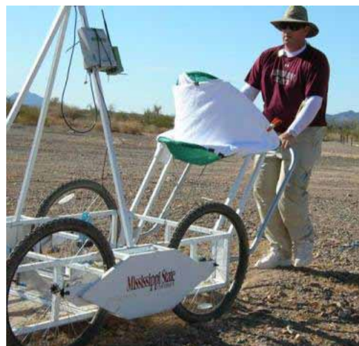
Figure 6. Radiation survey conducted by Mississippi State University using a push cart system (Etheridge et al. 2009).
