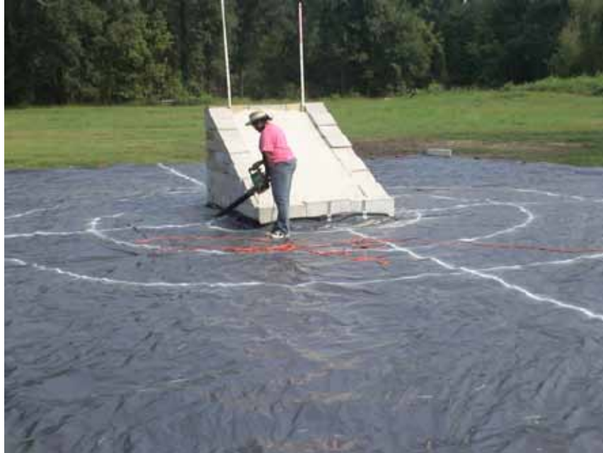
Figure 13. Catch box with sectors on the plastic tarp.
