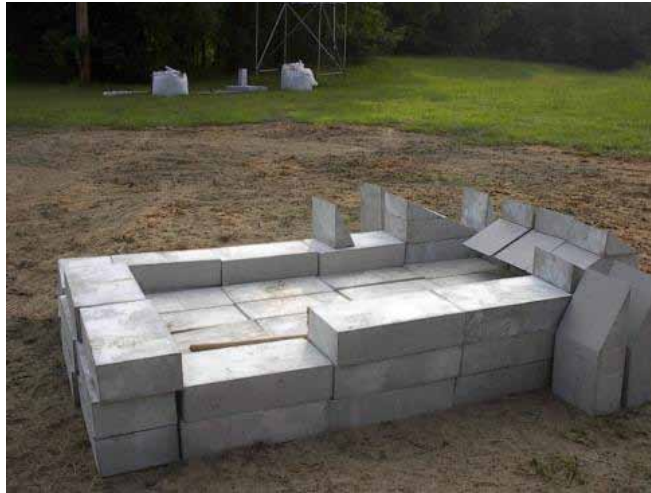
Figure 10. SACON® blocks used to create simulated catch box floor.
