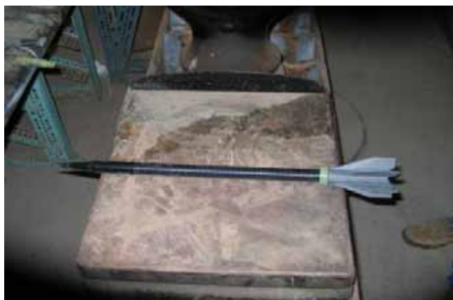
Figure 1. An M829 Class DU penetrator at Yuma Proving Grounds.
