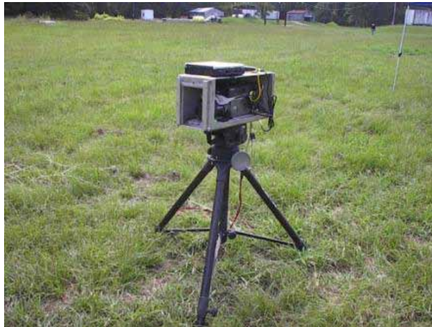
Figure 16. A tripod-mounted, high-speed Phantom camera.
