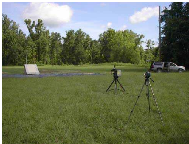
Figure 17. Set-up of Phantom and digital video cameras.
