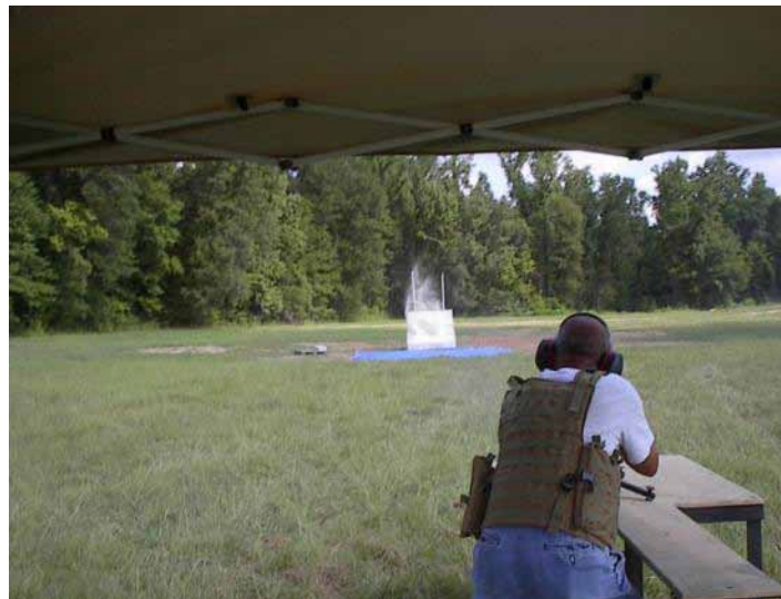
Figure 20. Impact of 50-caliber projectile into catch box from firing position.
