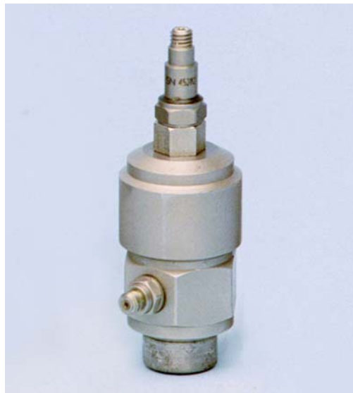
Figure 3 The PCB 301AO3 acceleration standard (bottom) with a PCB ICP ® accelerometer attached (top)
