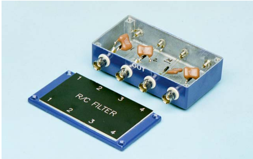
Figure 7 A box containing four simple, 26 kHz lowpass RC filters
