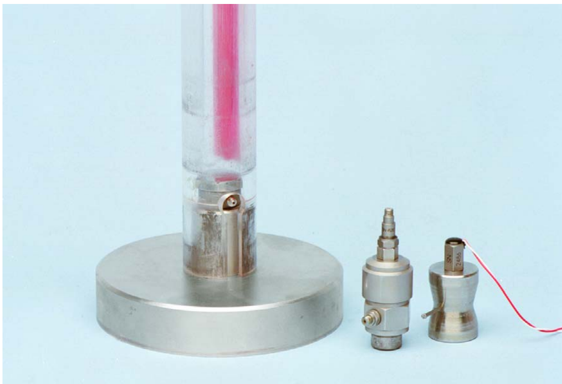
Figure 5 The Kistler force transducer with Perspex drop tower attached. The acceleration standard and a drop weight are shown each with a PCB accelerometer attached at the top.
