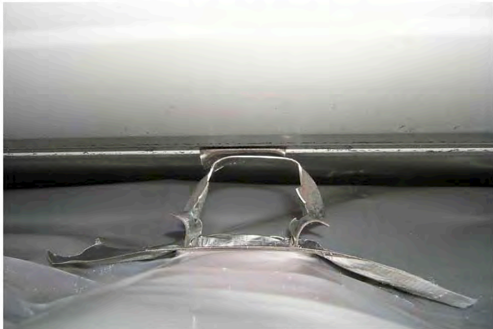
PHOTOGRAPH 12 EXPANSION CLIP FAILURE
