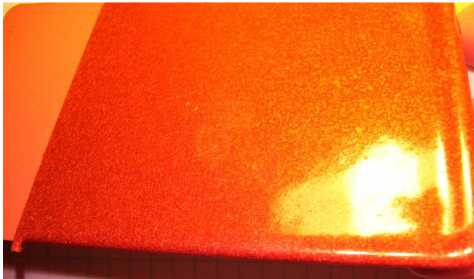
Figure 29. Gloss appearance of topcoating on test coupon.
