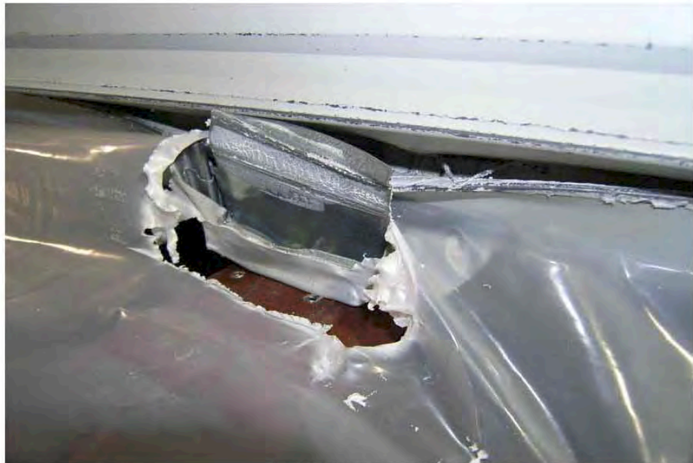
PHOTOGRAPH 22 FIXED CLIP FAILURE - 3
