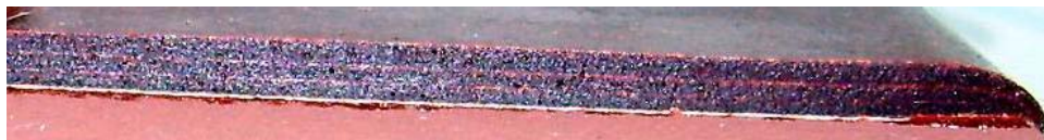
Figure 30. Distinct coating layers visible in cross section.
