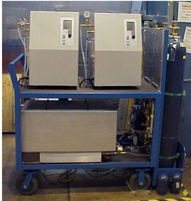
Photograph #2. SEOS 6 slpm cylinder fill breadboard as originally configured and tested at Air Products.
