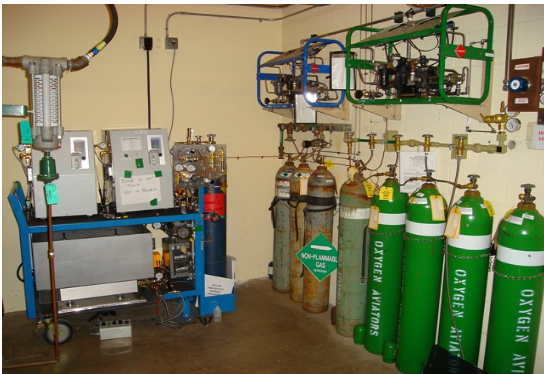
Photograph #4. SEOS breadboard shown with facility high pressure oxygen supply system.
