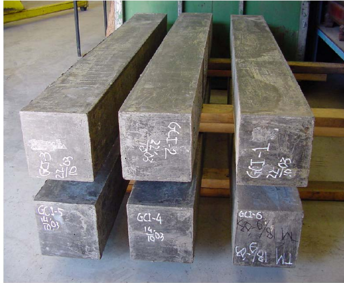
Figure 32. Geopolymer Columns After Demolding [52]
