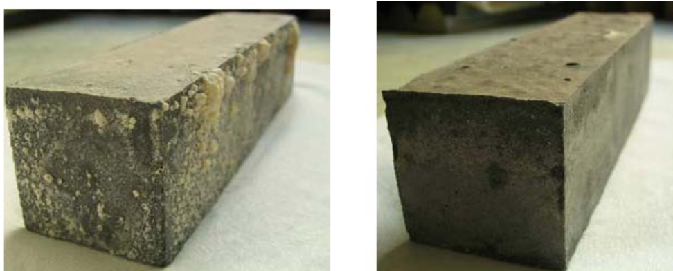
Figure 22. Geopolymer Mortar After 1.5 Years Exposure to \text{MgSO}_4 and \text{NaCl} Salt Solutions [6]
