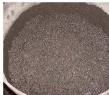
Figure 2. Fresh Geopolymer Concrete [4]
