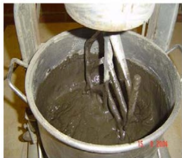
Figure 1. Fresh Geopolymer Binder Paste [4]
