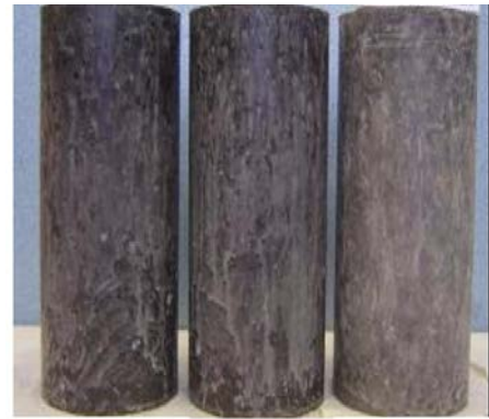
Figure 28. One-Year Visual Appearance of Geopolymer Specimens Exposed to [l-r]: 5% Na 2 SO 4 ; Fresh Water; Ambient Condition [45]
